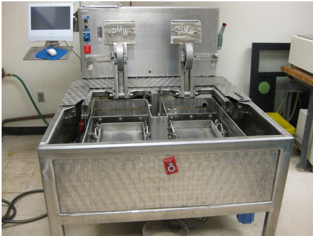
Figure 3-7 Hamburg wheel-tracking machine
