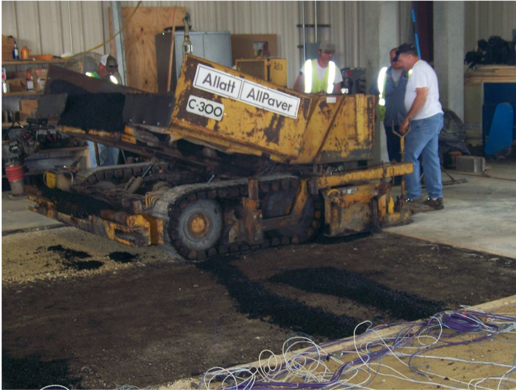
Figure 4-8 Lightweight asphalt paver
