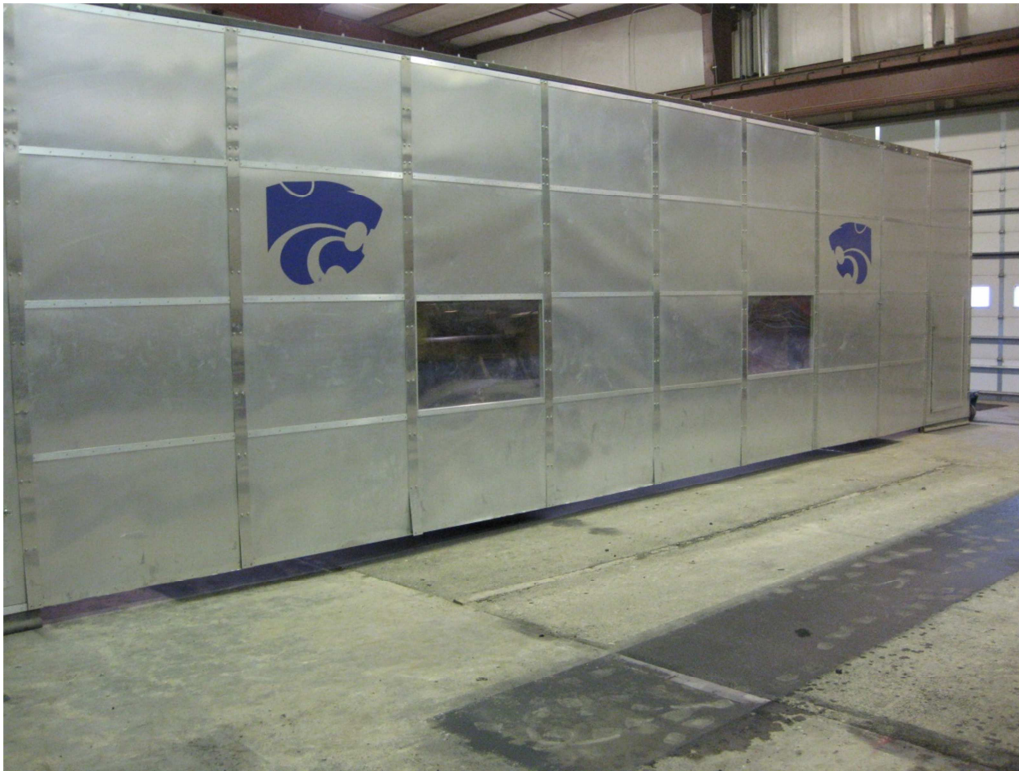
Figure 4-1 Environmental chamber around APT machine
