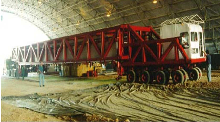
Figure 2-4 U.S. Army Corp of Engineers HVS (USACE 2011)
