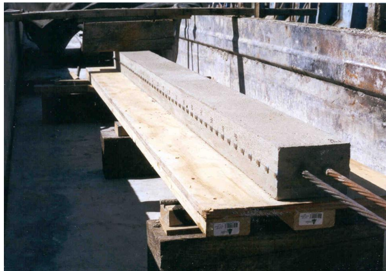
Figure 6-9 Metal points bonded onto the concrete surface
