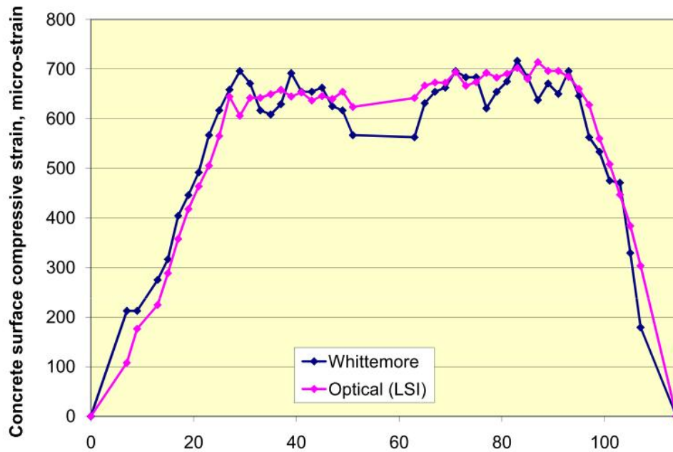
Figure 6-12 Comparison of strain measurements immediately after de-tensioning of a pre-tensioned specimen
