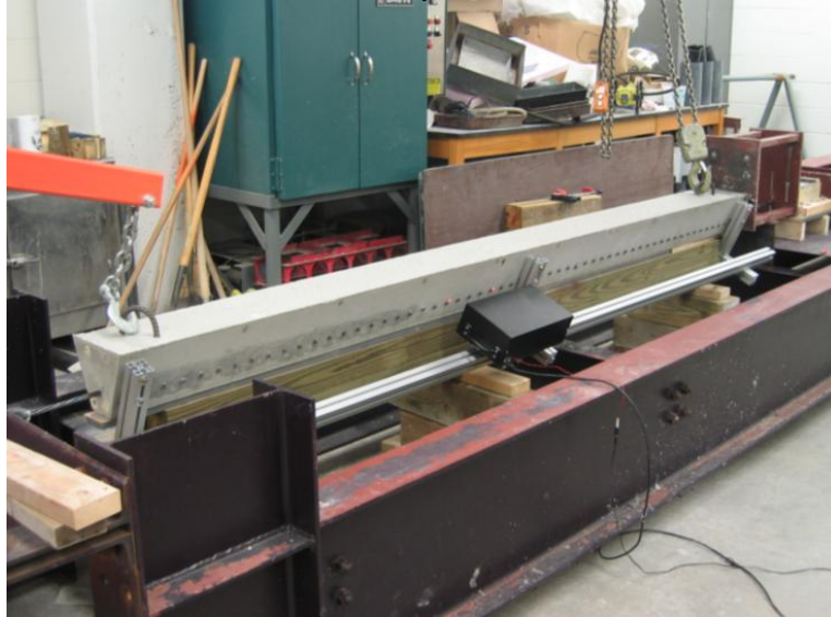
Figure 6-11 Experiment setup for transfer length measurement of prestressed concrete member using the second generation prototype
