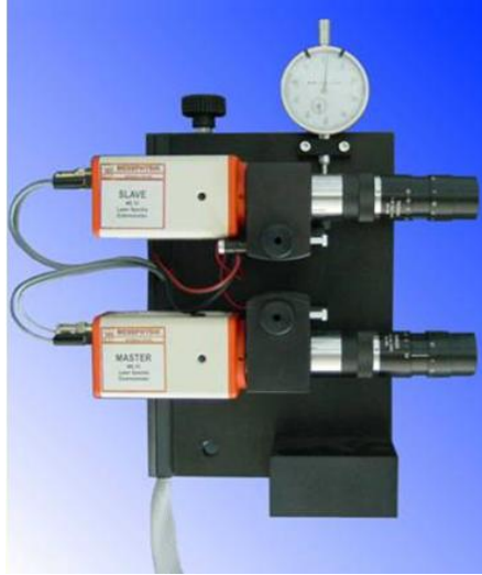
Figure 5-9 Messphysk company's laser speckle extensometer ME53-33
