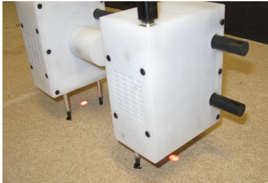
Figure 3-20 Visible markings and supporting legs used as the alignment mechanism
