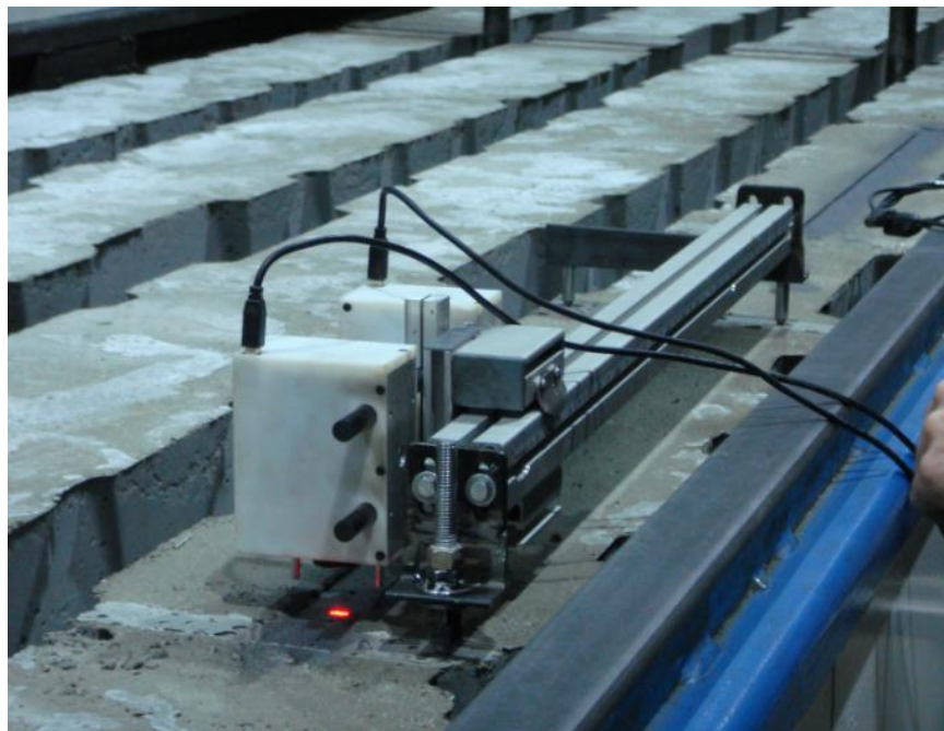
Figure 6-16 Laser speckle strain sensor mounted on a rail at CXT concrete cross-tie plant
