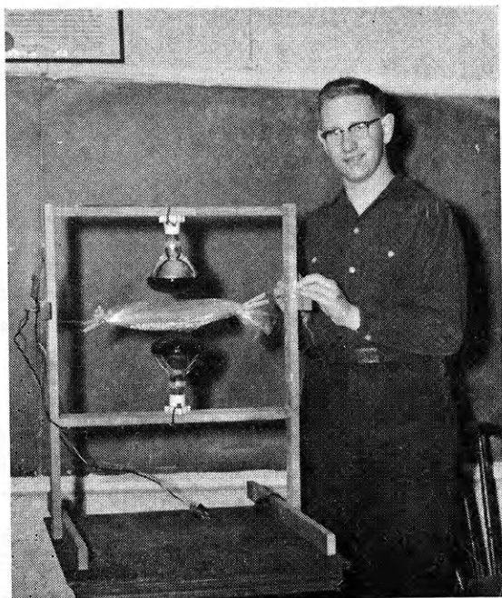
Carl Nichols, Lucky Diamond 4-H Club in Anderson County, demonstrates a popcorn popper he made in his 4-H Farm and Home Electric project. Two heat lamps pop the corn, which is suspended between them.
