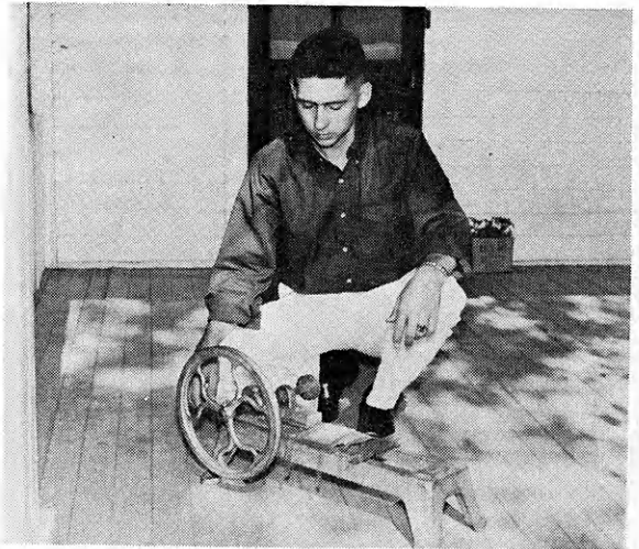
Ronnie built this speed reducer allowing use of an electric motor on an ice cream freezer. The whole family enjoys this.
