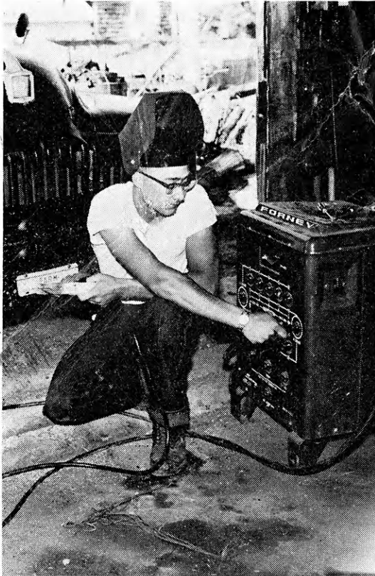
Making his own roof jack from a pipe, Bernard ran electric service to the farm work shop.
