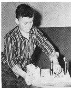
Here is the bright and dim switch Billy made for demonstration purposes. The difference in resistance of the two coils gives the bright or dim lighting effect.
