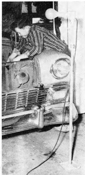
Billy received a blue ribbon at the County Fair last fall for his telescoping trouble lamp. Graduated rods were used for the stem so the lamp could be raised or lowered to the desired height.
