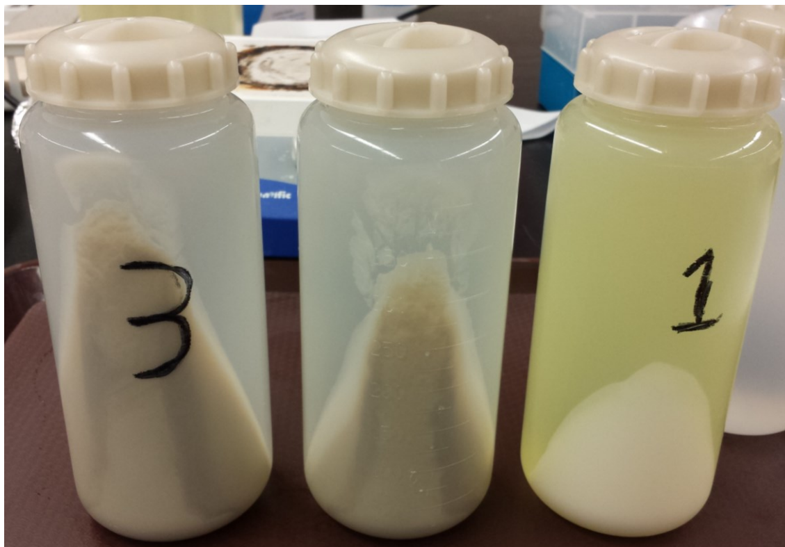
Figure F.2 Image of Color Change in Greek Yogurt Whey Top Aqueous Layers from Sepiolite Addition for Chapter 3; from left to right: centrifuged samples of 4g sepiolite per 100g Greek yogurt whey (GYW), 2g sepiolite per 100g GYW, and 0g sepiolite per 100g GYW
