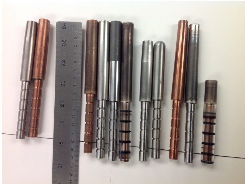
Figure 4.3: (Up) The machine stainless steel anode and six brass cathode rods supported on the brass base. (Down) Fabricated anodes for the KSU-DPF machine test. From the left side: Two stainless steel and copper semi tapered anodes, four Copper, stainless steel, graphite head, and Tungsten-copper (75/25) alloy straight anodes, two short semi-tapered and round head stainless steel anodes, two full tapered copper and stainless steel anodes, short straight Tungsten-copper (75/25) alloy straight anode.
