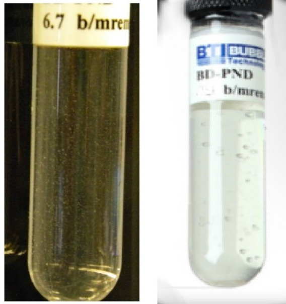
Figure 4.12: BTI neutron bubble detector of 6.7 bubble/mrem; the figure shows the detector before and after irradiation.
