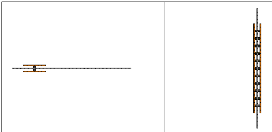
Figure 3.34: Mesh for sandwich panel with extended one column scatterers with retaining plates with scatterer diameter (D) of 1", lattice constant (B) of 3" and the length of scatterer (LS) of 2" (side views)
