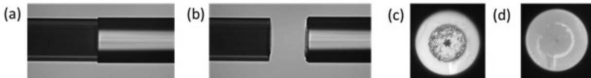
Figure 5-10: Splice image before and after the pull test. (a) side-view of a conventional splice of 10 \mu\text{m} PBGF (HC-1550-02) and SMF-28; (b) side-view after pulling test, the two fibers are pulled apart until breaking, the recorded pulling distance is 160 \mu\text{m} . (c) end-view of 10 \mu\text{m} PBGF after pull test; (d) end-view of SMF-28 after pull test.
