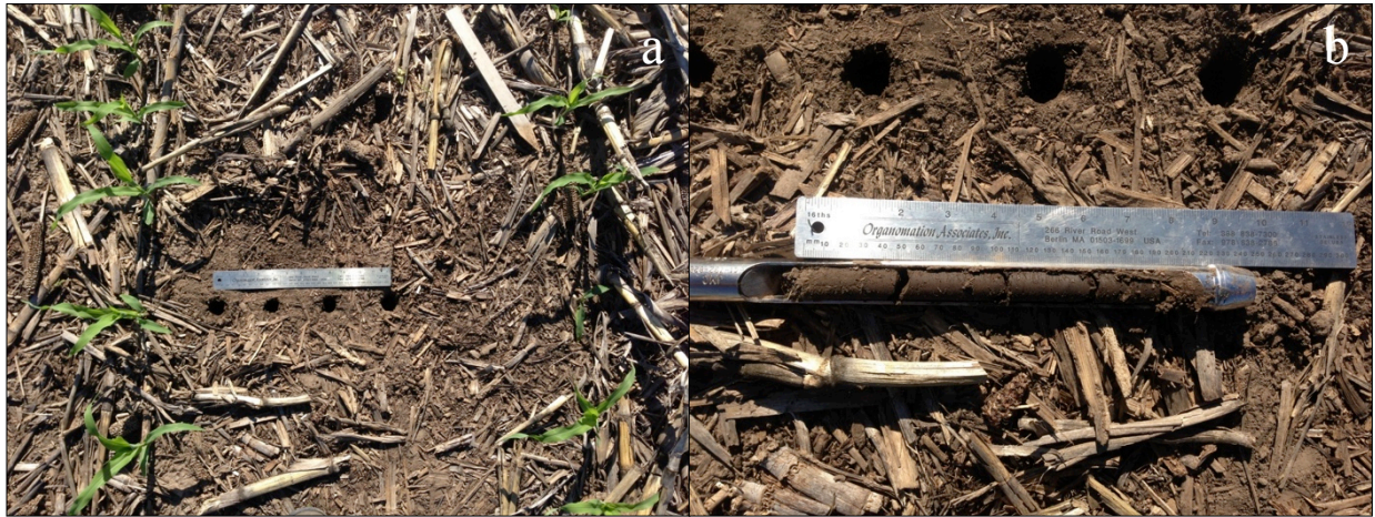
Figure 2.3. 2D soil sampling scheme. a) Locations 0, 10, 20 and 30 from right to left. b) Soil core partitioned in 0-5, 5-10 and 10-15 cm depths.
