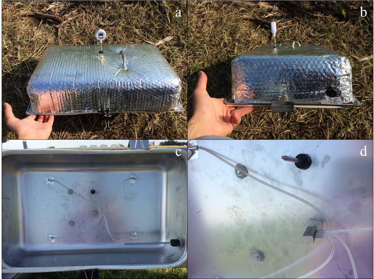
Figure 2.2. Chamber top a) in front view showing sampling port and thermometer, b) on a side view showing vent outlet, c) on an inside view showing vent tube, manifold and tubing branching to each quarter of the chamber, and d) a close up at the manifold.
