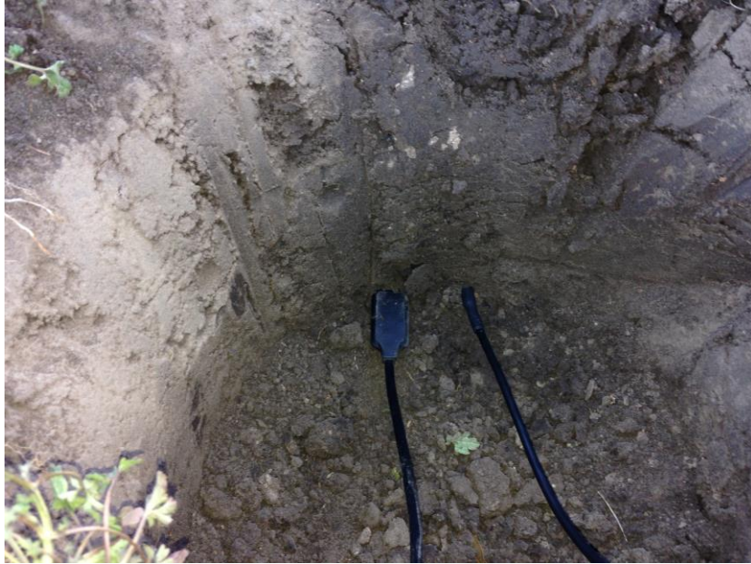
Figure 3-7. Soil moisture and temperature sensor placed at 10 cm.
