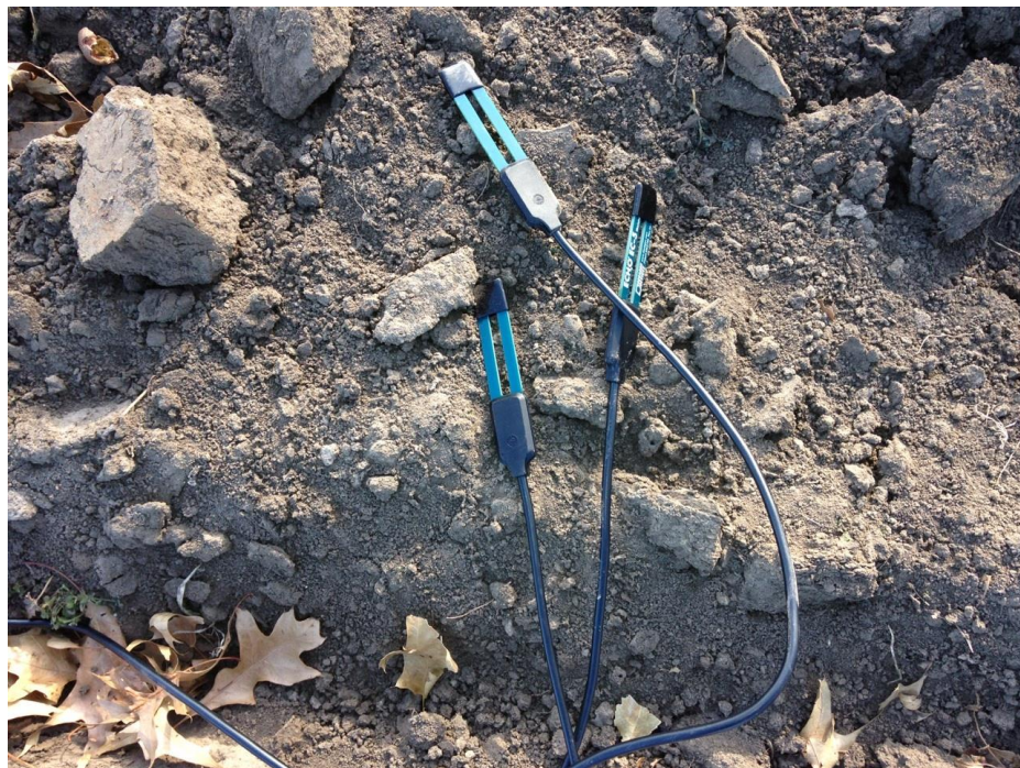
Figure 3-6. Dielectric soil moisture sensors used with HOBO weather station to record volumetric moisture content of the soil.
