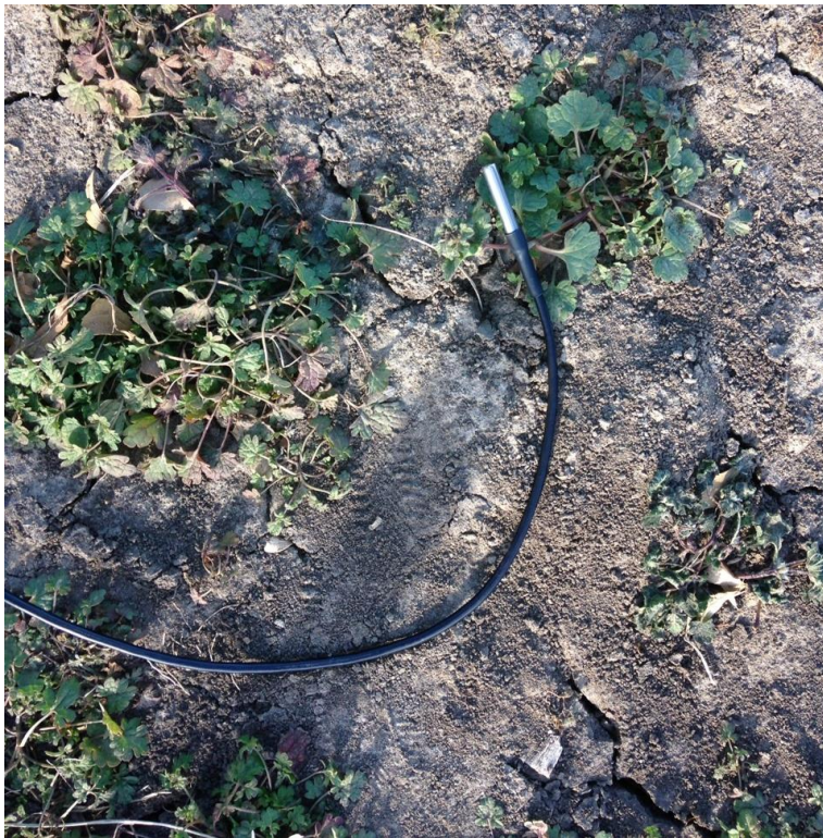
Figure 3-8. Temperature sensor used in recording soil temperature with HOBO mini data logger.
