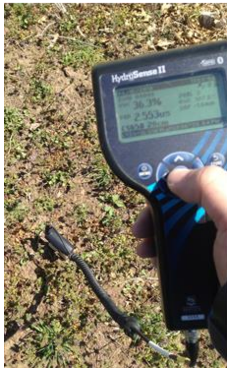
Figure 3-4. Campbell Scientific HydroSense II used to measure volumetric water content.
