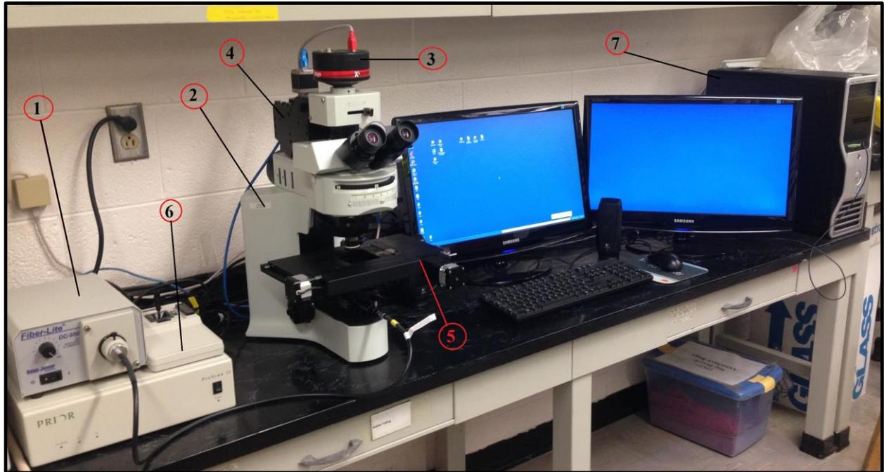
**Figure 5.2 CytoViva® Hyperspectral Imaging Microscope System. 1: Halogen light source; 2: Optical microscope; 3: Optical Camera; 4: VNIR spectrophotometer; 5: Motorized stage; 6: Controller for stage; 7: Computer**
