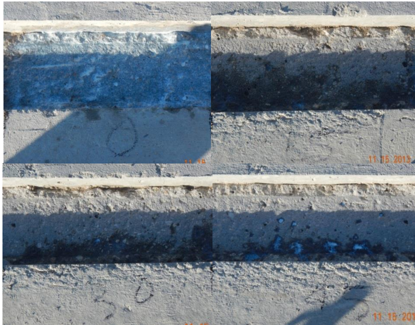
Figure 4.15 0, 15, 30, and 45 Minutes after Acrylic Bonding Agent Application
