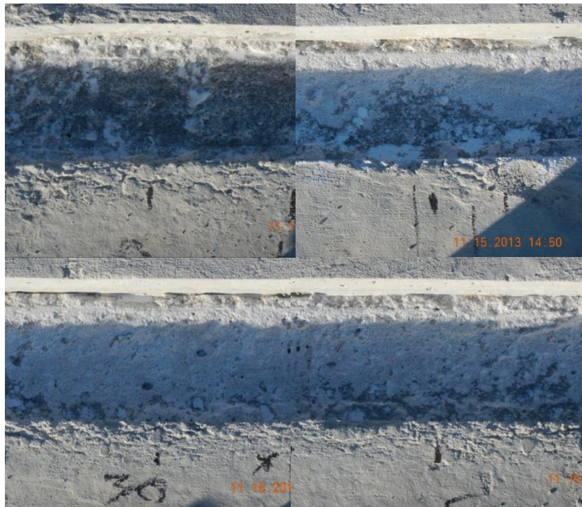
Figure 4.14 0, 15, 30, and 45 Minutes after PVA Bonding Agent Application
