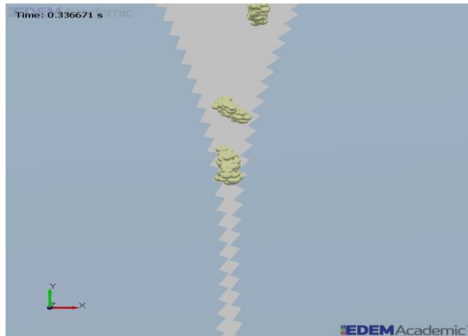
Figure 5-9: Size reduction by compression and shearing
