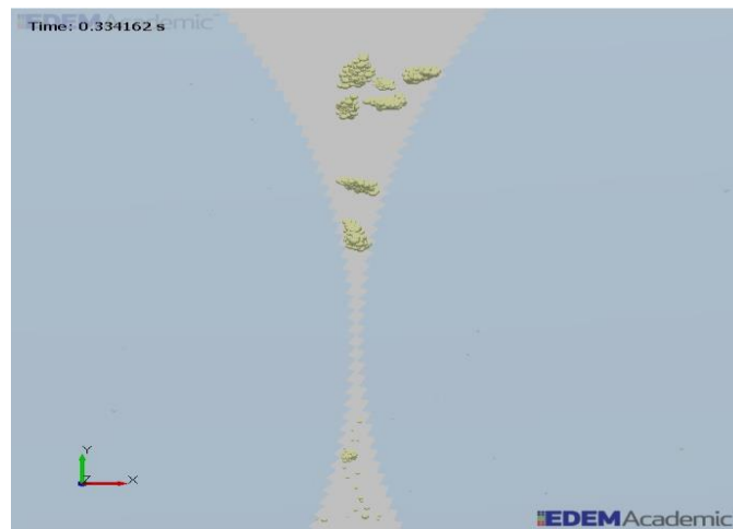
Figure 5-8: Bonded cluster passing through the rolls during milling process
