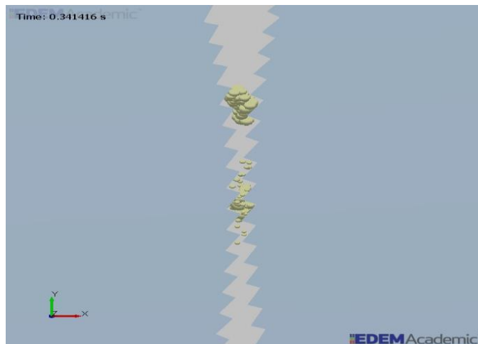
Figure 5-10: Breakage of cluster into smaller particles
