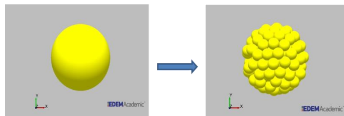
Figure 4-4: Replacement of whole particle by cluster of fraction particle using particle replacement factory.
