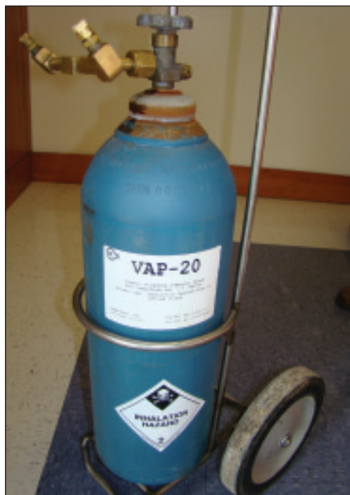
Shown here is a typical pressurized cylinder that is holding the aerosol dichlorvos (Vapona). Photo courtesy of Dr. Bhadriraju Subramanyam (Subi).
