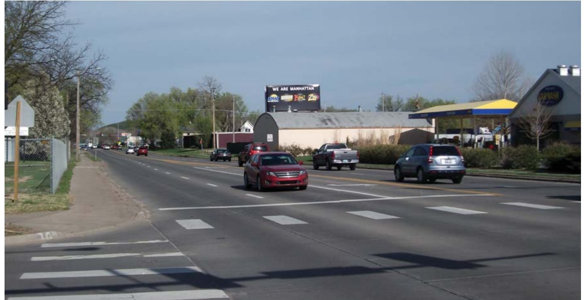
Fig. 4. FORT RILEY BOULEVARD Long crossing distances and lack of pedestrian facilities.
