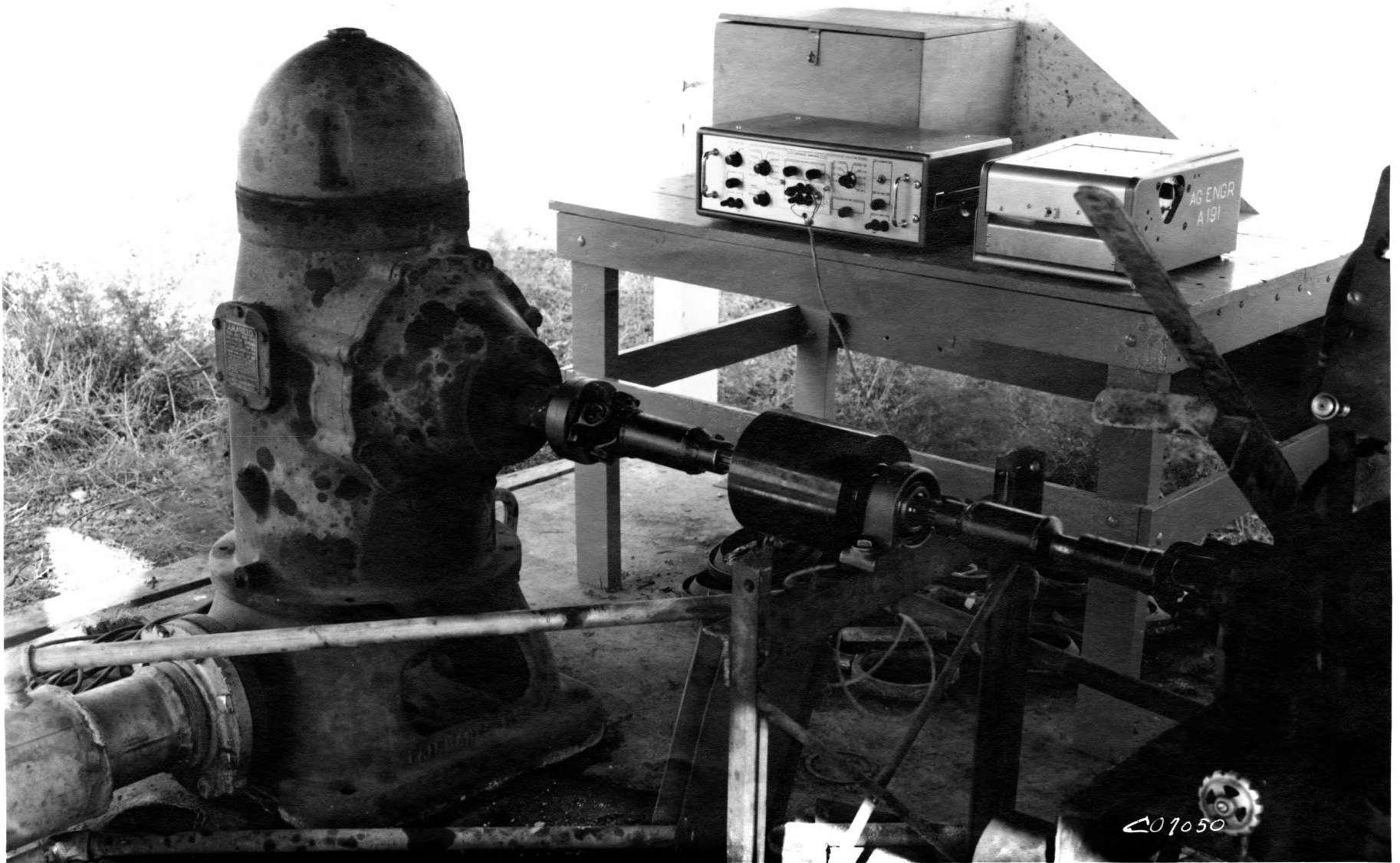
Fig. 16. The torquemeter installed between an irrigation pump and its power source.
