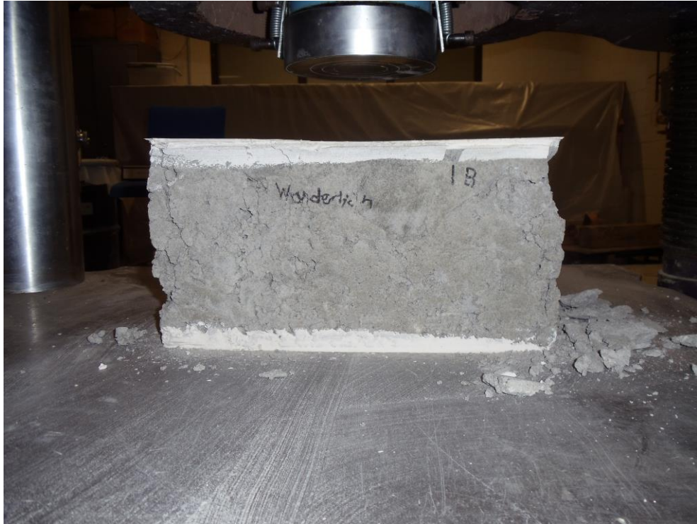
Figure 6.1 Specimen 1B Failure
