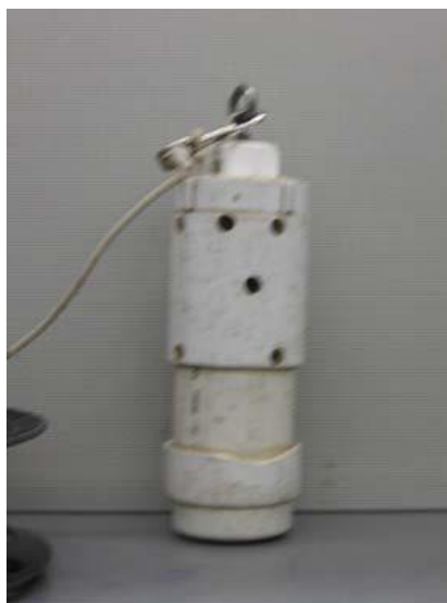
Figure 3.8 Water sampling device (Reproduced from Steele, K.L. 2008. Atrazine best management practices: Impact on water quality. MS thesis. Manhattan, KS: Kansas State University, Department of Biological and Agricultural Engineering.)
