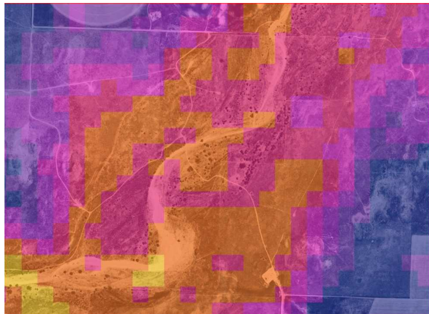
Figure B15: Depth to Groundwater, in m, at Study Site 5 in (a) 1965 and (b) 2005.
