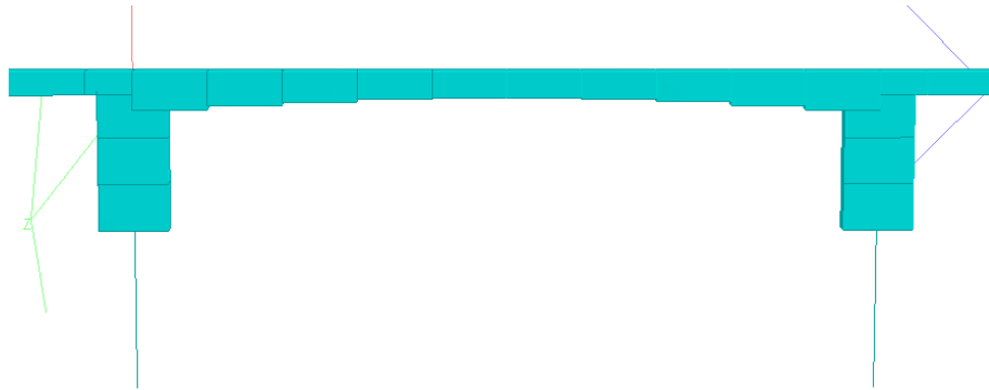
Figure 3.4: Stepped Member Offsets Shown in STAAD Model
