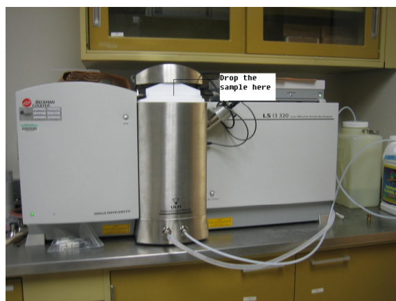
Figure 2.3 Image of a LS™ 13 320 Laser Diffraction Particle Size Analyzer with Universal Liquid Module
