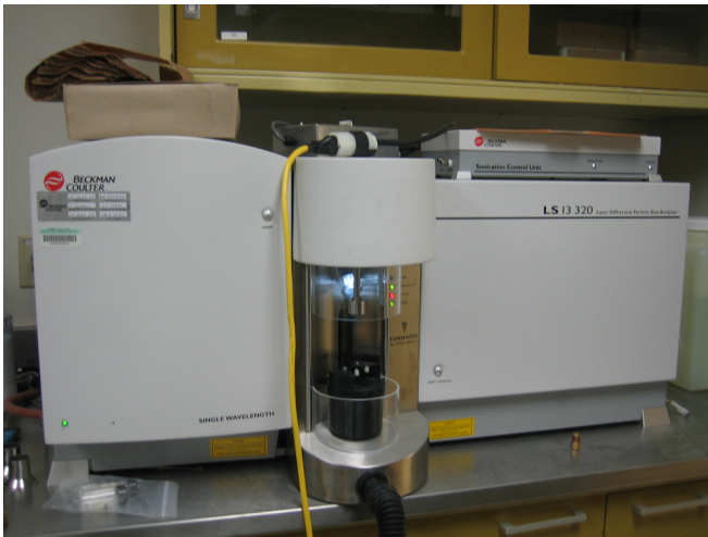
Figure 2.4 Image of a LS™ 13 320 Laser Diffraction Particle Size Analyzer
