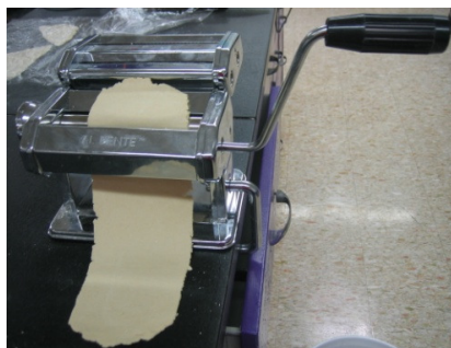
Figure 3.2 Image of sorghum noodle sheeting process
