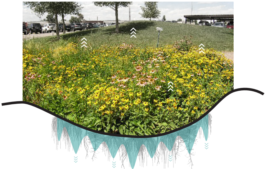
Figure 33: Rain Garden Diagram. Diagram by author. Adapted from United States Environmental Protection Agency, 2013.
