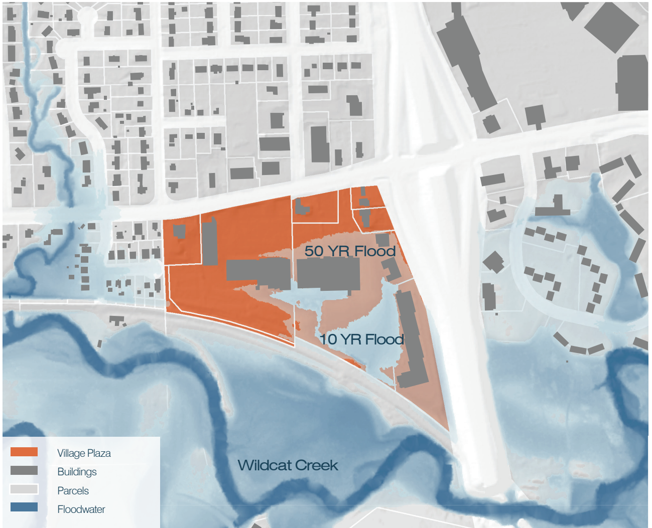
figure 6.26 - Village Plaza Flooding
