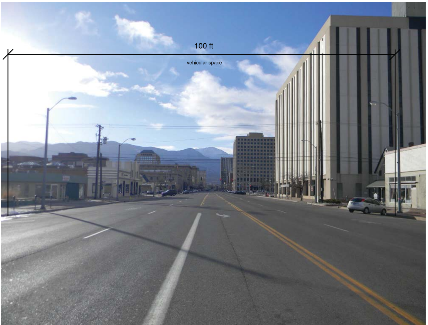
Figure 1-3. View of the wide, automobile-oriented street of Pikes Peak Avenue. While the entire right-of-way measures approximately 140 feet, vehicular lanes and parking take up 100 feet of space (photo by Devin Ash)
