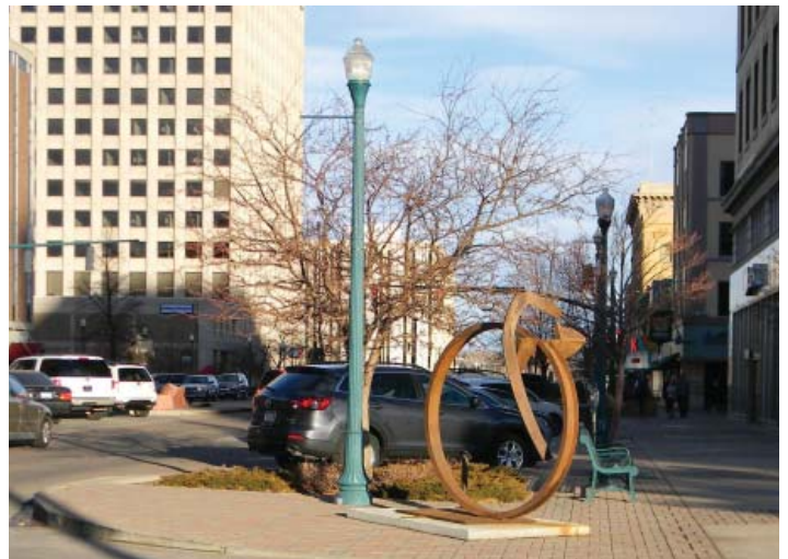
Figure 3-22. Pedestrian bump out with seating, lighting, street trees and public art (photo by Devin Ash)
