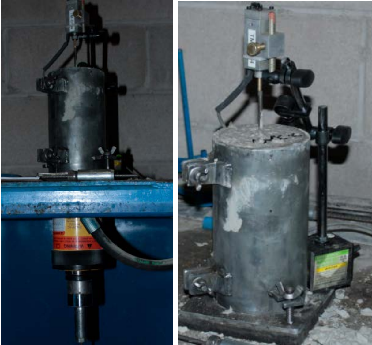
Figure 6.6 a) Specimen in testing machine at CXT and b) LVDT on specimen at CXT
