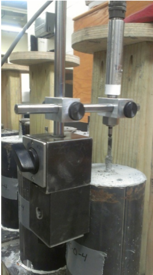
Figure I.3 LVDT and magnetic base setup used for test development
