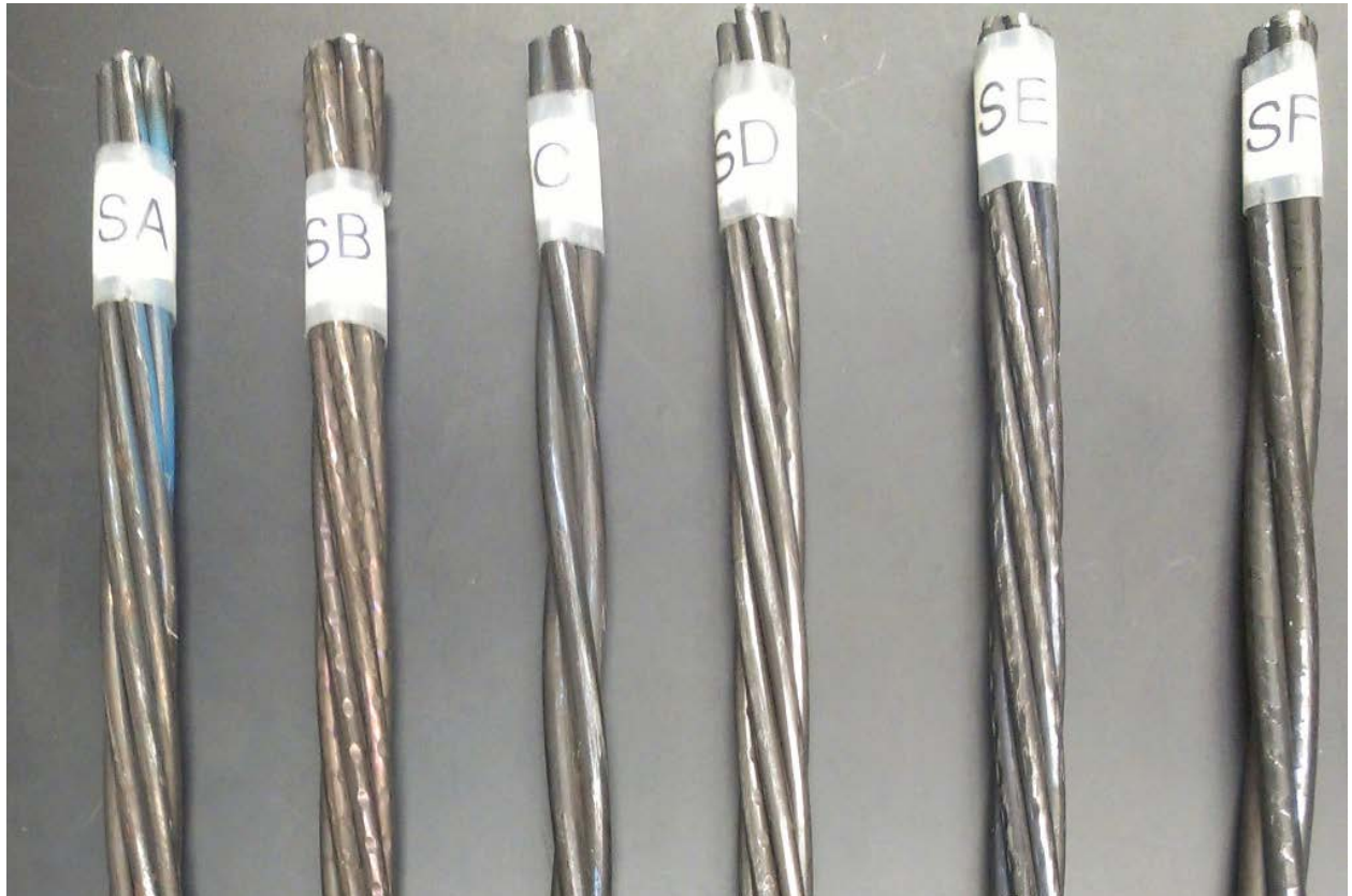
Figure 3.3 Sample of the six strands with various indent geometries and diameters
