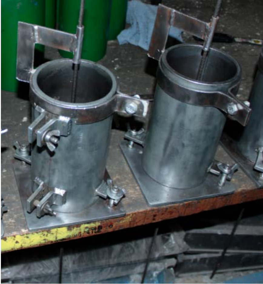
Figure 6.3 Additional fixture used to center reinforcement during casting at CXT
