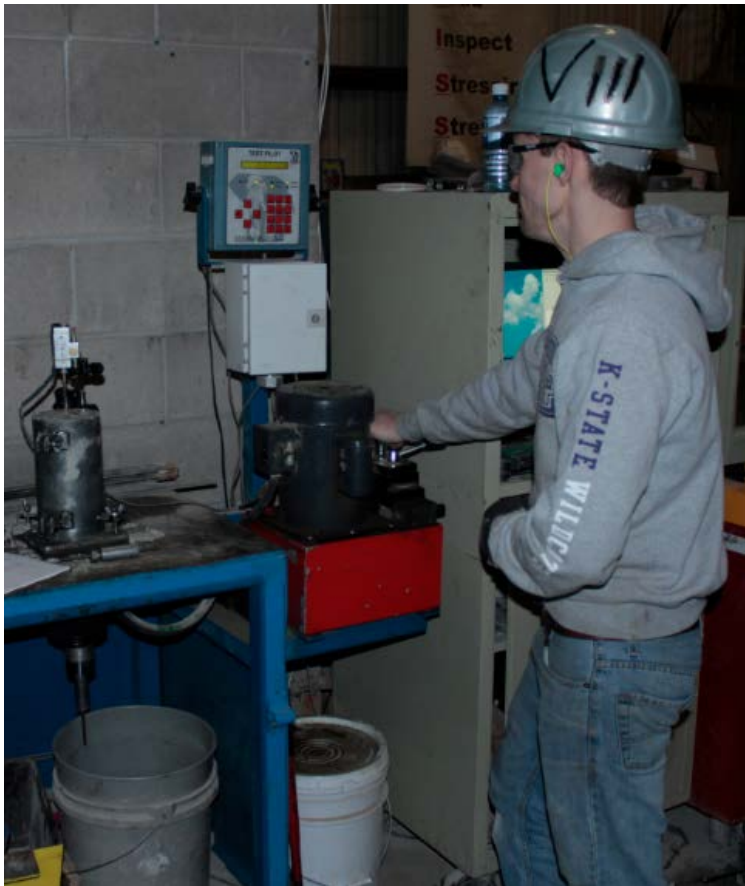
Figure 6.5 Manually controlling force loading rate at CXT
