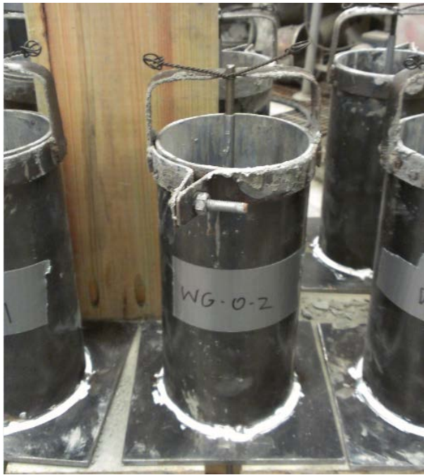
Figure 4.15 Additional fixture used to center reinforcement during casting
