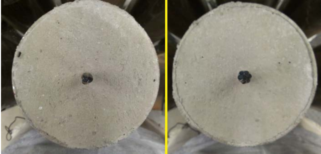
Figure 5.6 Top view of three-wire and seven-wire strand specimens
