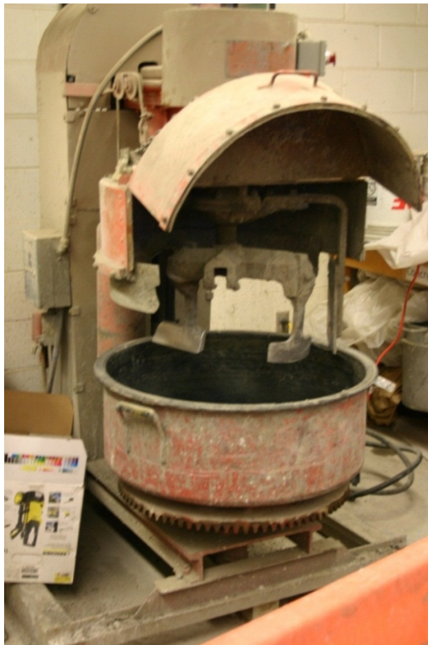
Figure 4.17 Pan mixer used for wire pullout tests
