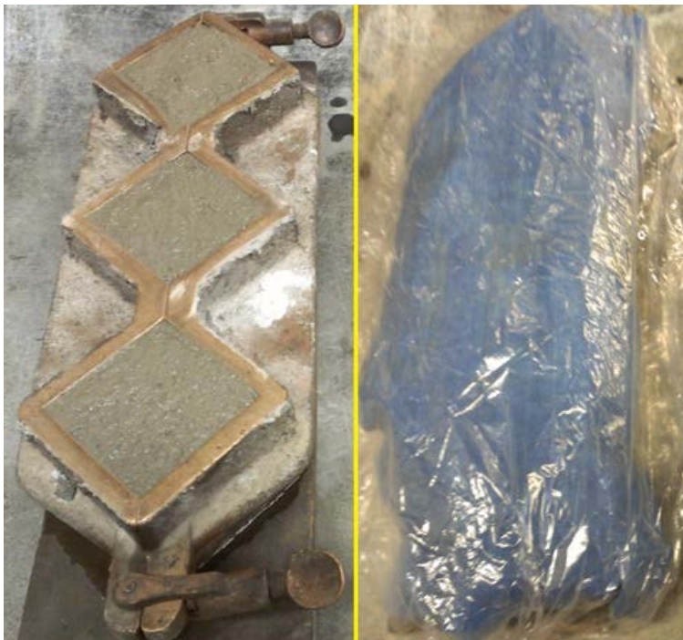
Figure 4.19 2-in. mortar cubes uncovered and covered
