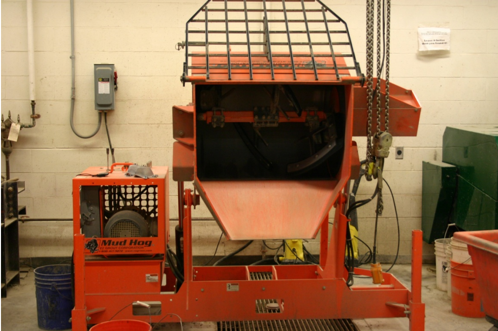
Figure 5.5 Paddle mixer used for strand pullout tests
