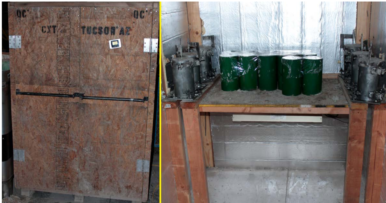
Figure 6.4 Outside and inside of temperature-controlled storage closet at CXT
