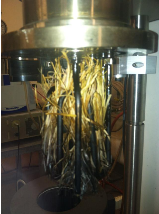
Figure 5-1: Pre-Dried CRP Torrefaction (250 °C, 30 min.)
