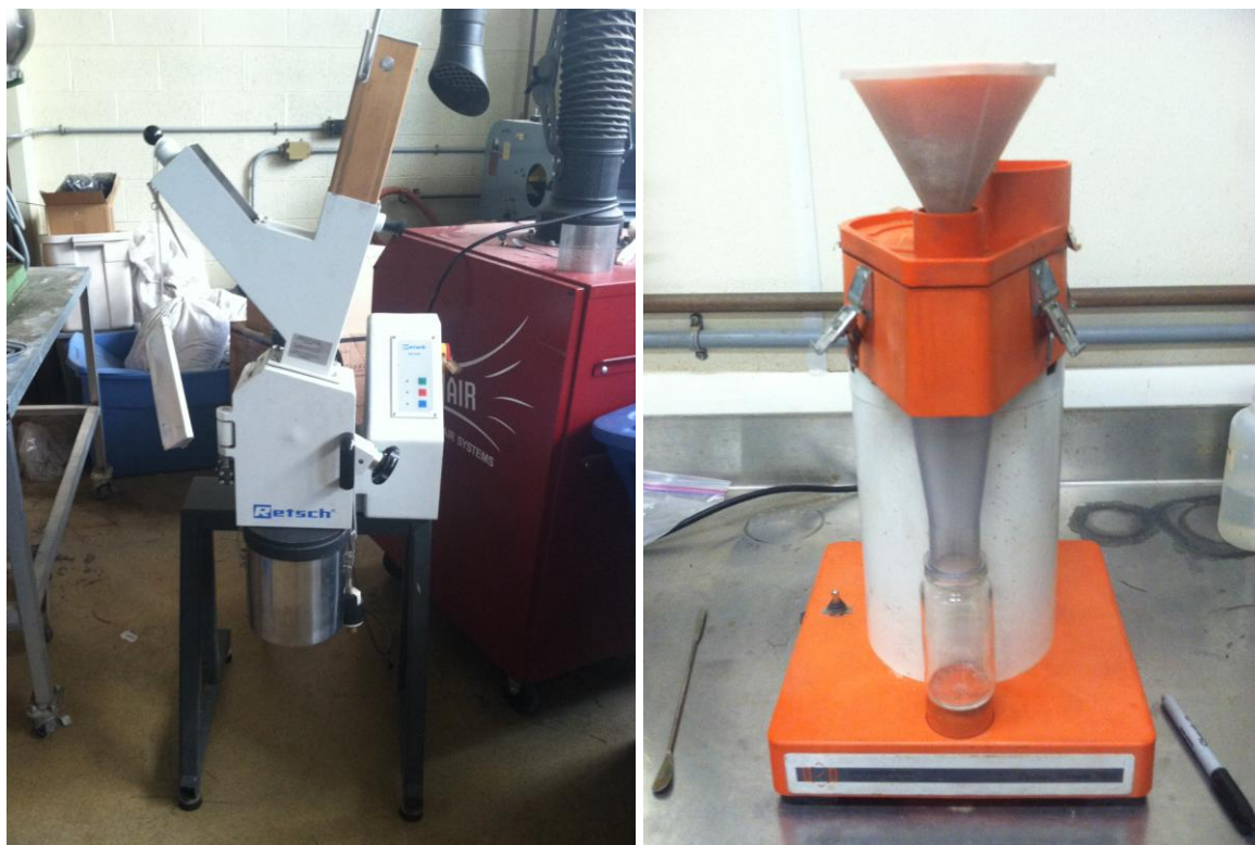
Figure 4-4: Retsch SM 2000 Grinder / UDY cyclone mill
