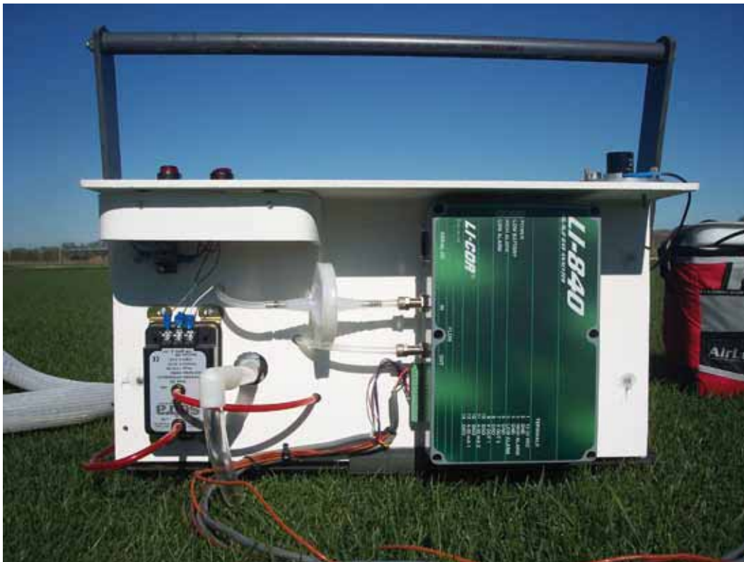
Figure 2. The chamber console included a closed-path infrared gas analyzer (Licor 840, Licor Biosciences, Lincoln, NE) and a pressure differential transducer.
