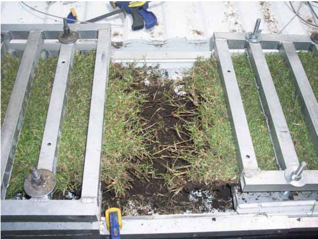
Figure 2. Sod was evaluated for tensile strength.
