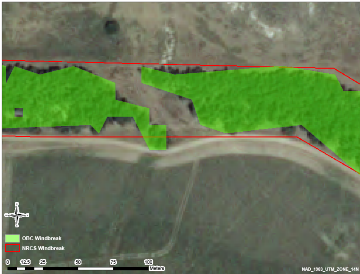
Figure 21. Example of a fragmented windbreak classified by NRCS as a single unit, but as two distinct units by object-based classification.
