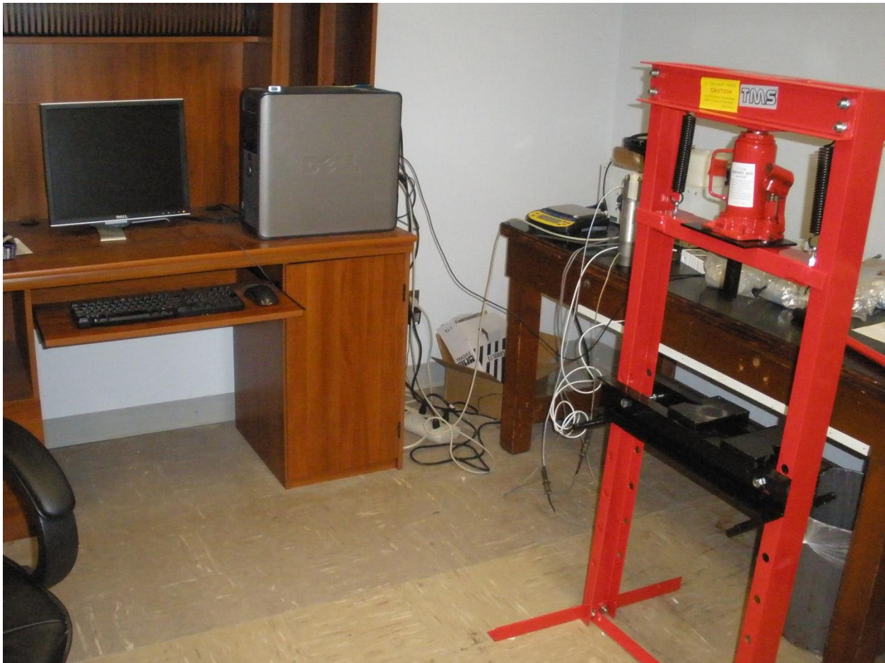
Figure 16 - ULT system and hydraulic press setup
