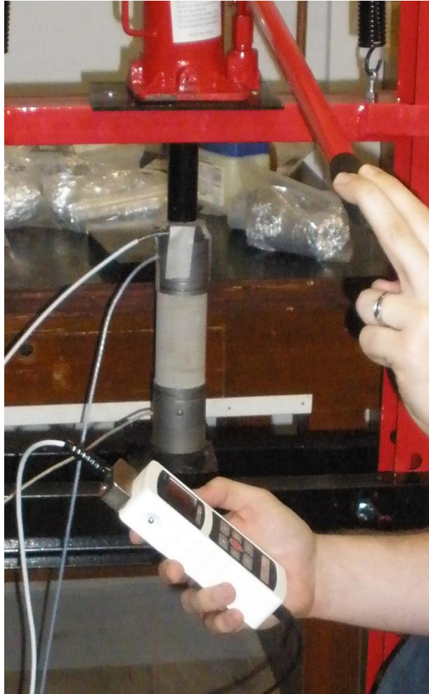
Figure 17 - Close up of core sample in hydraulic press while applying calculated overburden
