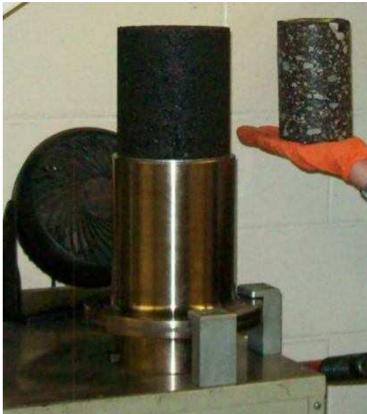
Figure 3.9 Superpave gyratory compactor sample, and cored and trimmed sample
