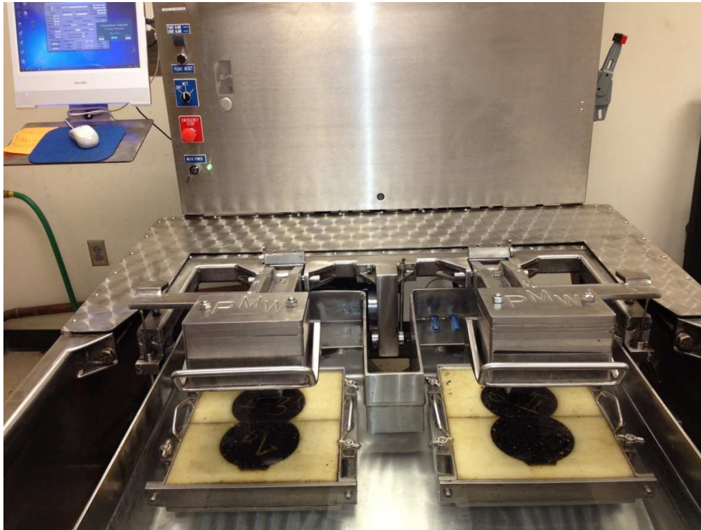
Figure 3.5 Hamburg wheel-tracking device (HWTD) test setup
