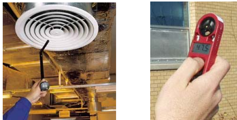
Figure 5.3: Velocity stick (left) and anemometer (right)
