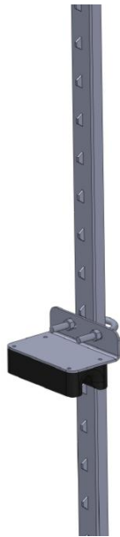
Figure 31. Fourth Generation Sensor Mounted on a T-Post
