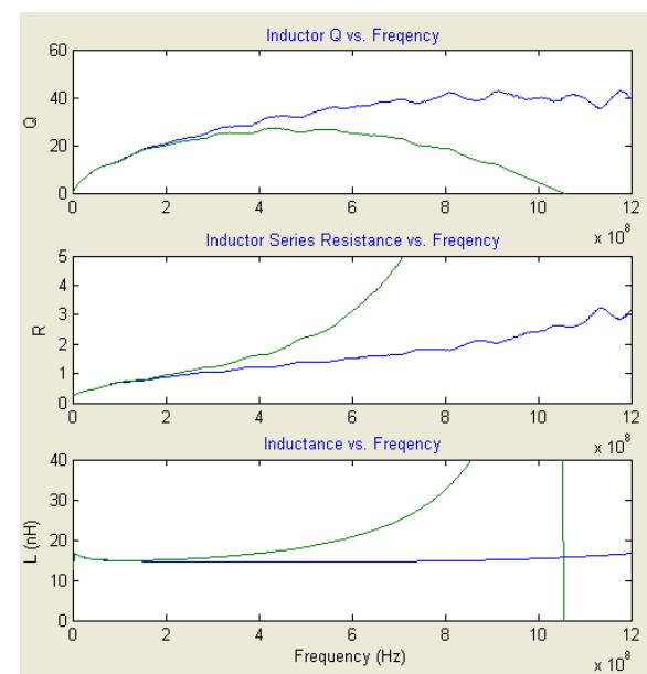
**H4: 3 TURNS, 18MIL PITCH, .5DIA SHIELD WIDTH,
