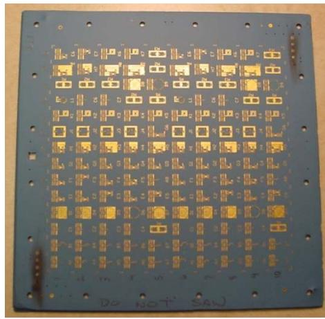
FIGURE 3.1: A PANEL OF THE INDUCTOR ARRAY
