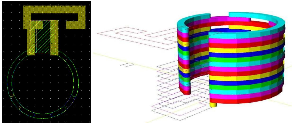
FIGURE 7.1: DEEP-LOOP RESONATOR
