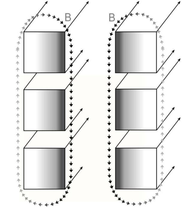
FIGURE 2.3: UNEVEN CURRENT DISTRIBUTION CAUSED BY SKIN EFFECT PLUS PROXIMITY EFFECT IN A SOLENOID.
