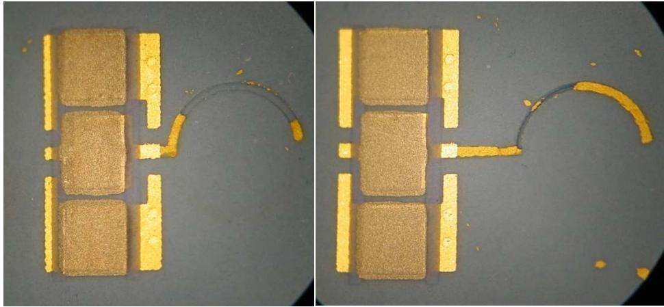
FIGURE 6.1: EXAMPLES OF UNFILLED TRENCHES ON TOP LAYER
