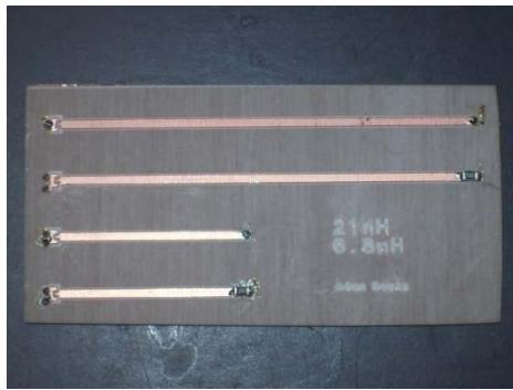
FIGURE 4.6: MICROSTRIP LINE USED FOR GAMMA CORRECTION
