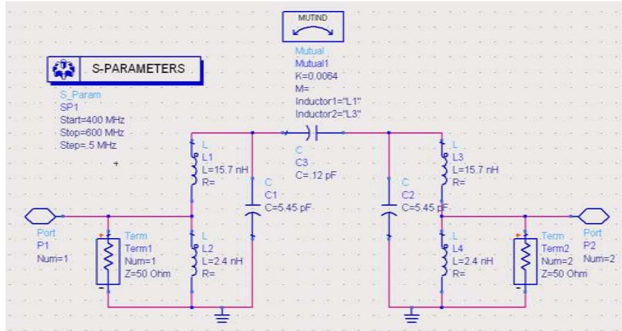
FIGURE 7.3: CONFIGURATION OF THE PROPOSED 2-POLE FILTER
