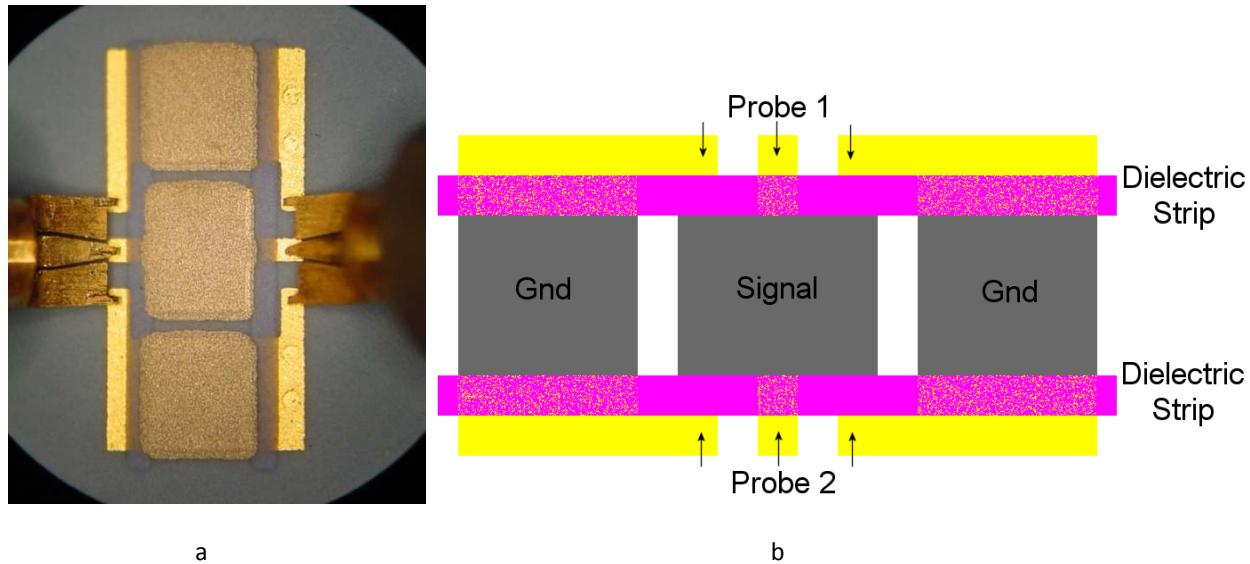
FIGURE 4.10: TOP SIDE PROBING STRUCTURE W/O CAPS
