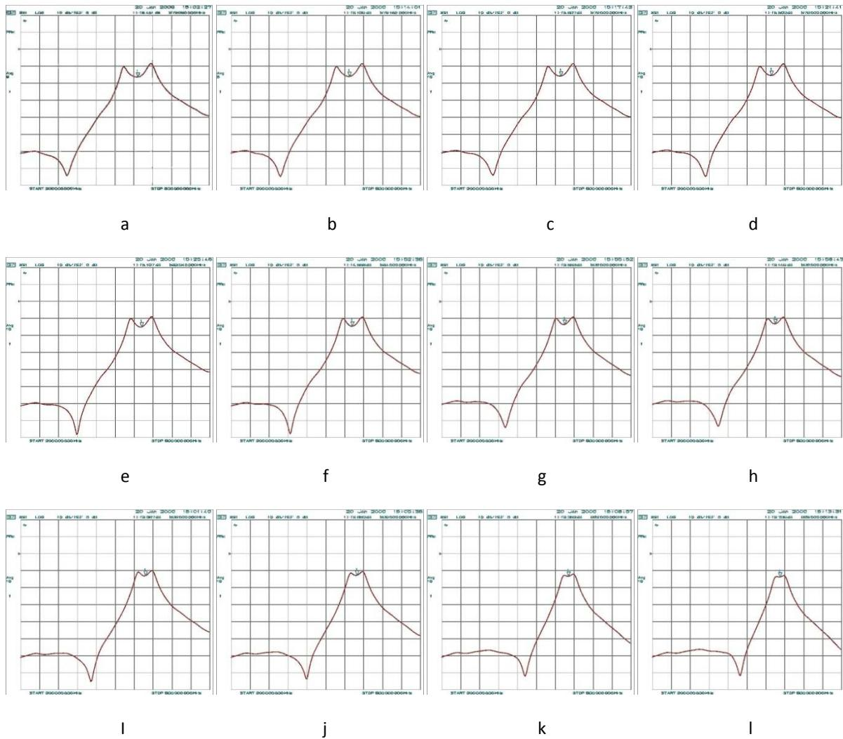
FIGURE 7.6: PROGRESSION OF 2-POLE FILTER RESPONSE AS COUPLING CAP IS TRIMMED
