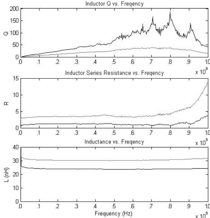
FIGURE 4.2: A SAMPLE OF TWO MEASURED INDUCTORS WHERE ONE INDUCTOR HAS A  $|\Gamma|$  NEAR 1.
