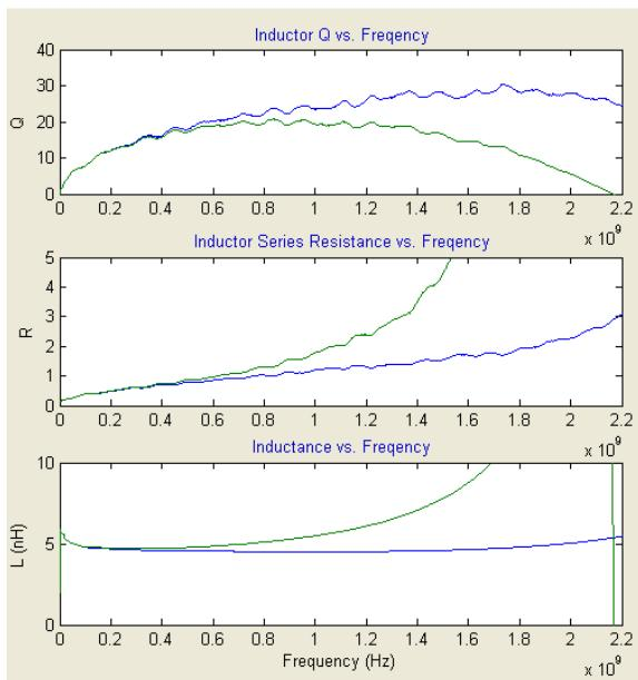
**H3: 6 TURNS, 12MIL PITCH, 1DIA SHIELD WIDTH,
