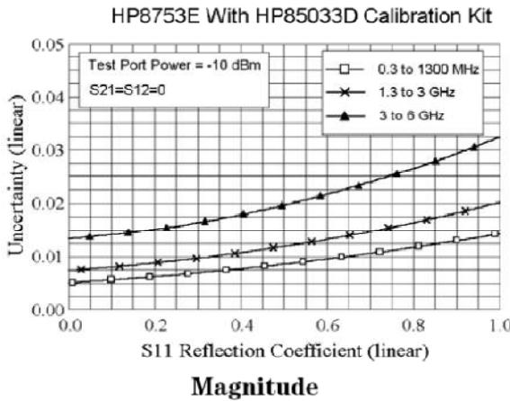
FIGURE 4.4: HP/AGILENT DATASHEET GRAPH OF SPECIFIED GAMMA MAGNITUDE ACCURACY (FROM AGILENT WEBSITE)
