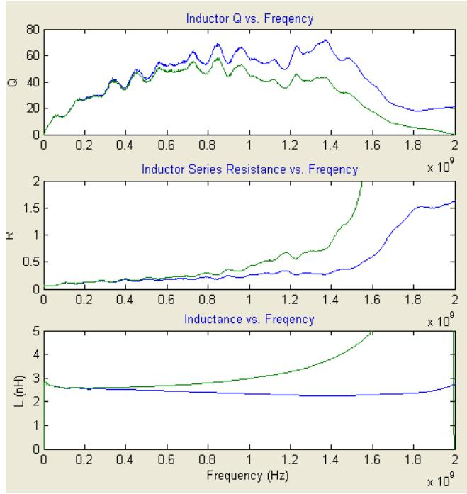
FIGURE 7.2: MEASURED RESULTS OF THE DEEP-LOOP RESONATOR
