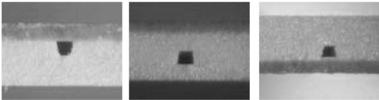
FIGURE 2.4: EXAMPLES OF LASER-CUT VIA CROSS-SECTIONS [15]
