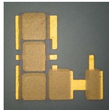
FIGURE 4.12: PROBING STRUCTURE WITH TOP SIDE SERIES CAP PAD
