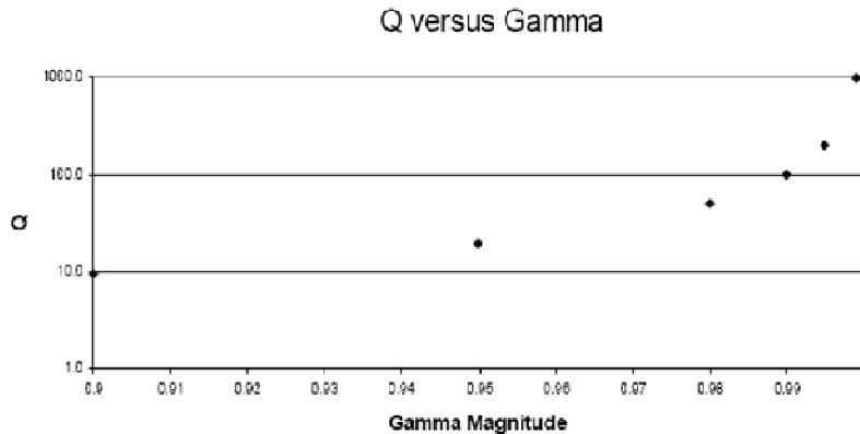
FIGURE 4.3: Q VERSUS GAMMA FOR BEST CASE MEASUREMENT (ANGLE GAMMA = 90 DEGREES)
