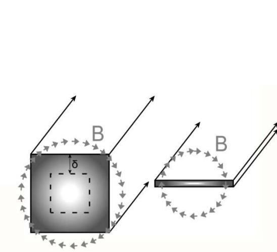
FIGURE 2.2: UNEVEN CURRENT DISTRIBUTION CAUSED BY SKIN-EFFECT. HERE, DARKER SHADING INDICATES A HIGHER CURRENT DENSITY.
