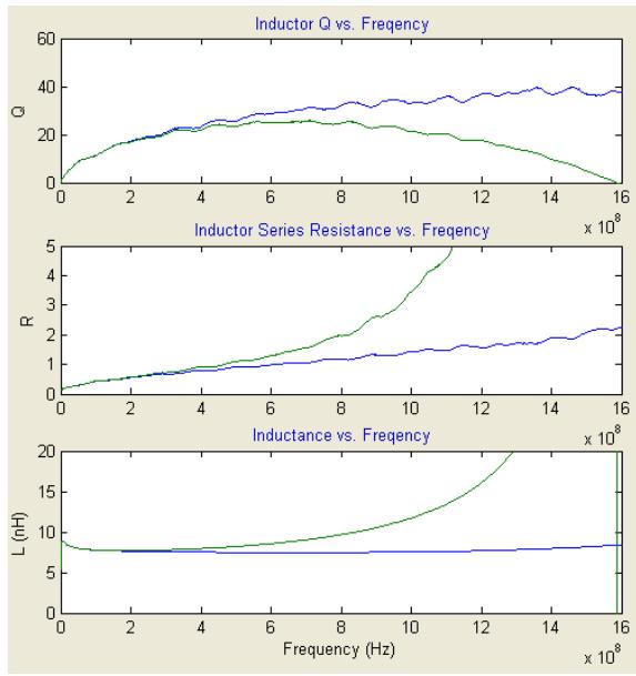
**H5: 6 TURNS, 18MIL PITCH, .5DIA SHIELD WIDTH,
