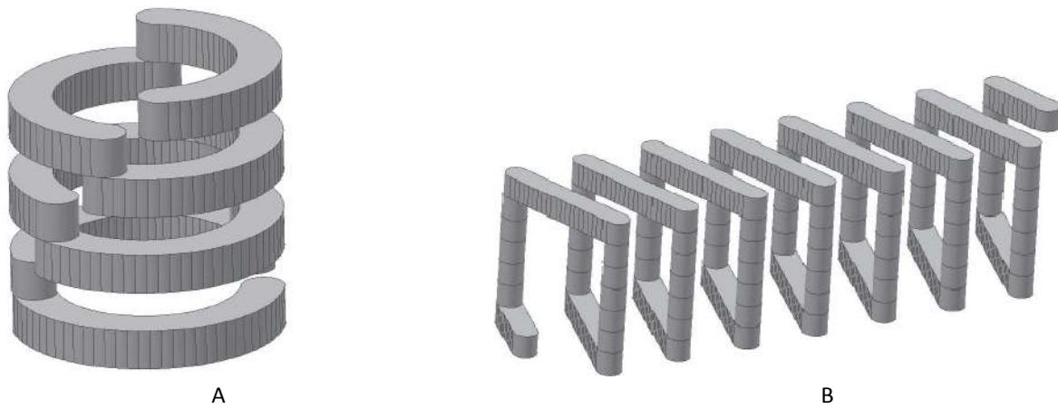
FIGURE 2.1: VERTICAL(A) AND HORIZONTAL(B) SOLENOIDS CREATED USING OVERLAPPING PUNCHED VIA STRUCTURE IN LTCC MATERIAL
