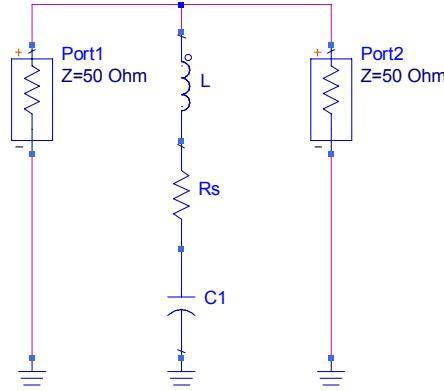
FIGURE 4.5: 2-PORT MEASUREMENT SETUP
