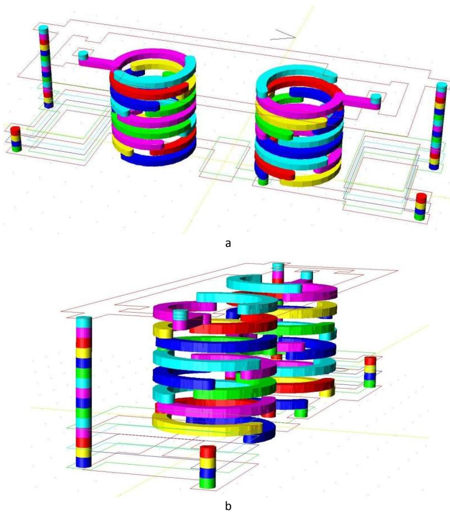
FIGURE 7.5: A FTTF 2-POLE FILTER. ALL 2-D FLAT METAL TRACES AND CAPACITORS ARE SHOWN AS OUTLINES.
