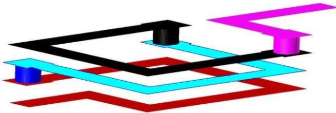
FIGURE 1.1: A TYPICAL HELICAL INDUCTOR MADE FROM THIN METAL TRACES.
