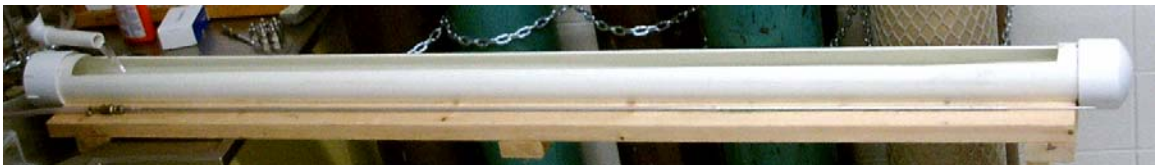
Figure 7.20: Long water tank used for leak checking each flux probe tube.
