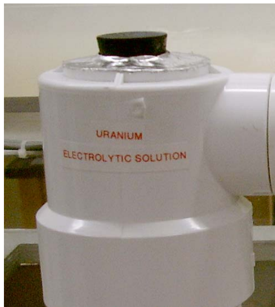
Figure 7.11: Sensor port for loading a pH and temperature sensor in the electrolytic flow path or for adding chemicals to the solution.
