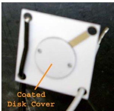
Figure 4.4: A different design trying to get good contact between the anode and cathode and their respective wires.
