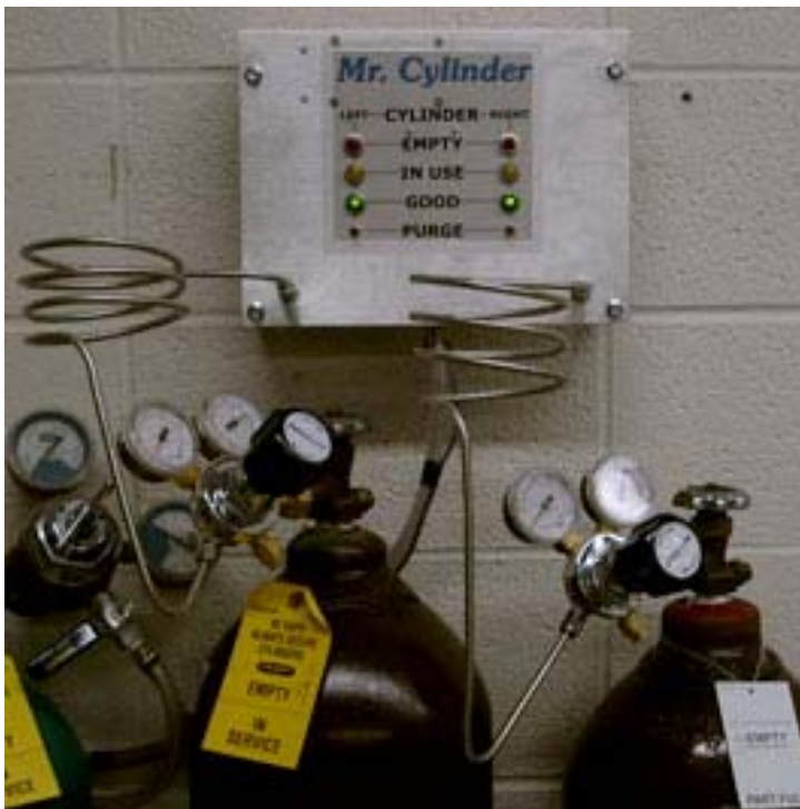
Figure 7.5: Mr. Cylinder system for automatically switching between argon gas bottles for the annealing oven.
