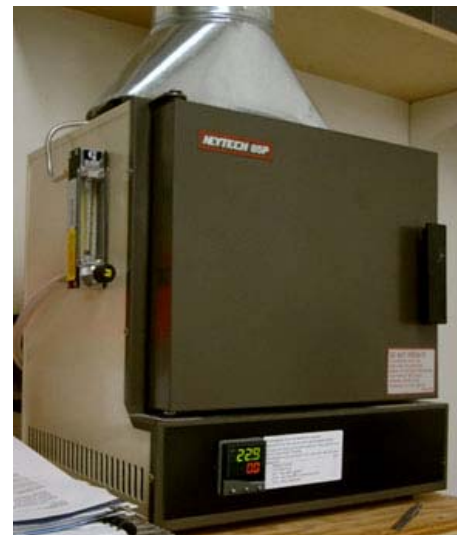
Figure 7.4: Nytech oven with new controller and inert gas injection line.
