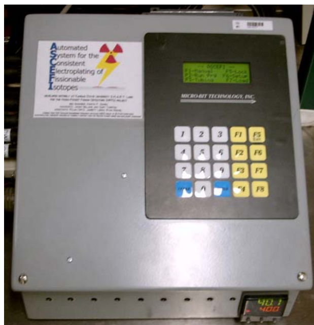
Figure 7.13: ASCEFI controller which monitors and controls all system components.
