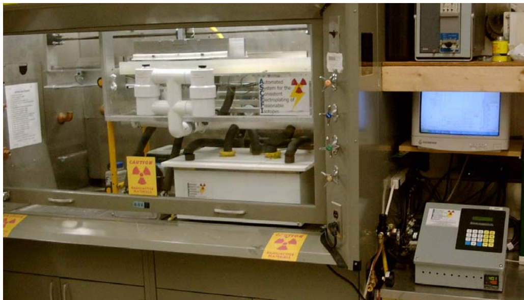
Figure 7.7: The Automated System for the Consistent Electroplating of Fissionable Isotopes. plating chamber, the hot water bath and electrolyte storage, the electrolyte flow subsystem, and the system controller.
