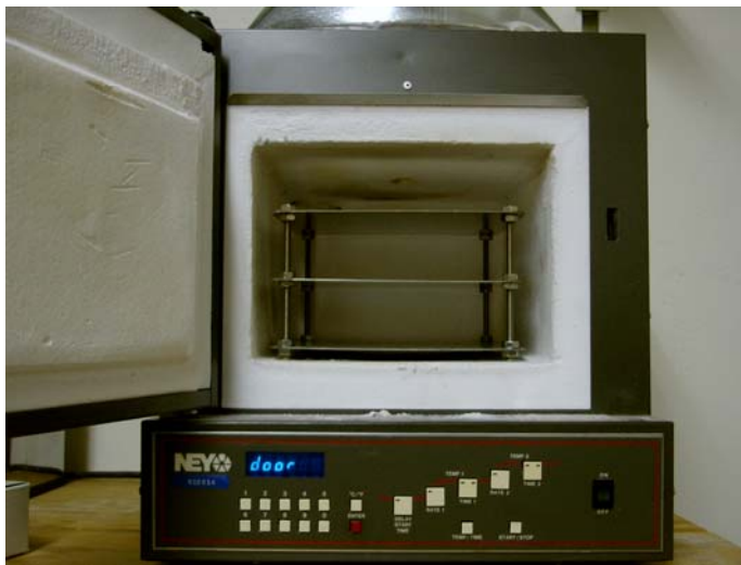
Figure 7.3: Nytech oven with old malfunctioning controller system. Internal area with new shelving shown.
