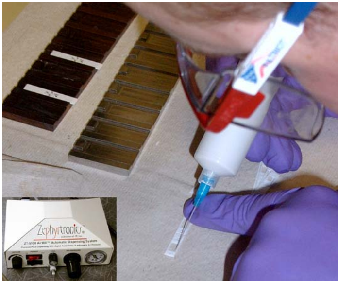
Figure 7.14: Application of the alumina epoxy using the Zephytronics Air Mill dispensing system.
