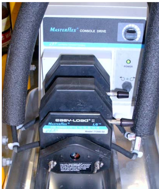
Figure 7.10: Peristaltic pump for controlling electrolytic solution flow.
