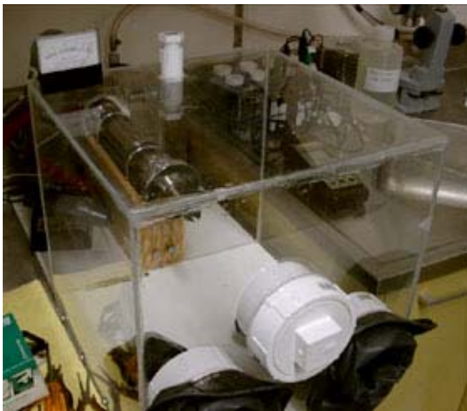
Figure 7.16: Custom built glove box and vacuum system for the back filling of the detectors with pure argon.
