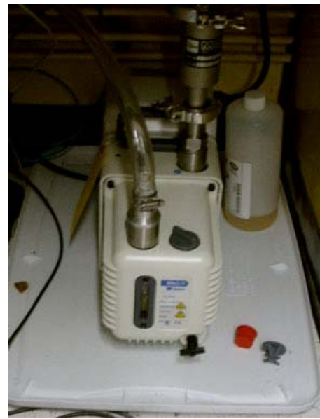
Figure 7.17: Direct drive rotary vane vacuum pump used in the backfilling system.
