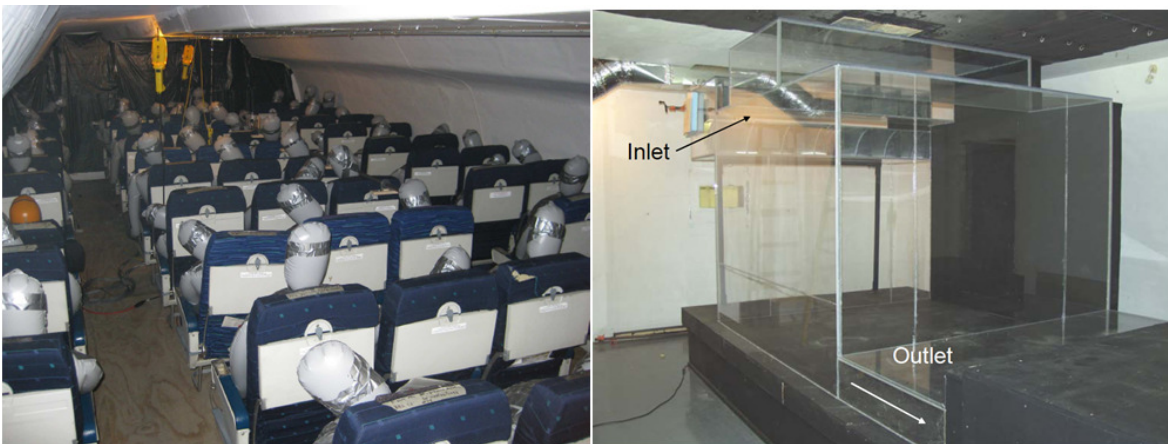
Figure 1.4: The full-size 11-row Boeing 767 cabin mockup (left) and the Boeing 767 generic cabin model (right)
