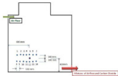
Figure 15: Points 1-14 are the sampling points above and below the injection tube. The concentration values of CO 2 are predicted using LES at these points and compared with the corresponding experimental data for CFD validation purposes.
