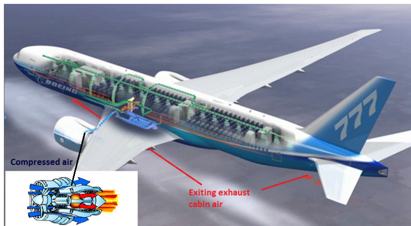
Figure 1.2: A view of a typical air-conditioning system for a commercial aircraft cabin. The picture shows how the compressed fresh air is drawn off the engine and mixes with the highly filtered cabin air in equivalent portions to provide appropriate cabin environment for normal breathing. The picture also shows the exhaust cabin air exiting the lower lobes of the fuselage (Boeing, 2011 and NASW, 2011).
