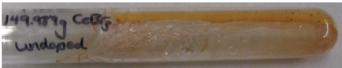
Figure 5.3. Ingot HB6, undoped \text{CeBr}_3 under normal light. Internal cracking prohibited harvesting useable samples.
