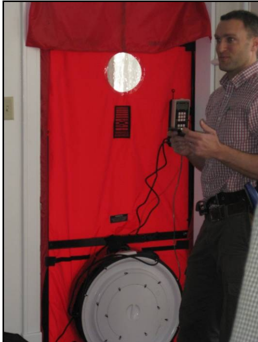
Figure 2.2 Chad Robinson Conducting a Blower Door Test
