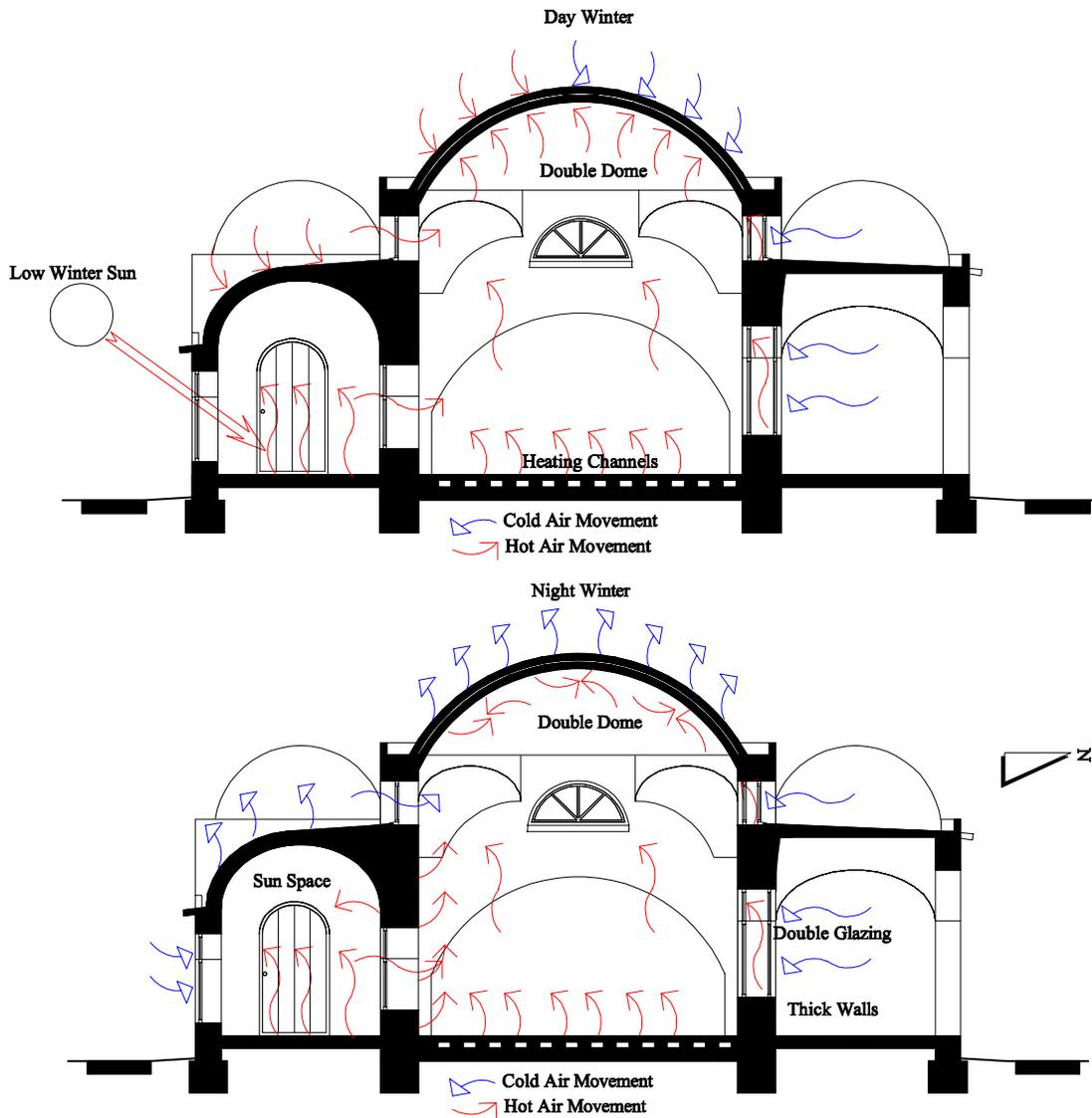
**FIG. 27 PASSIVE & ACTIVE HEATING**
