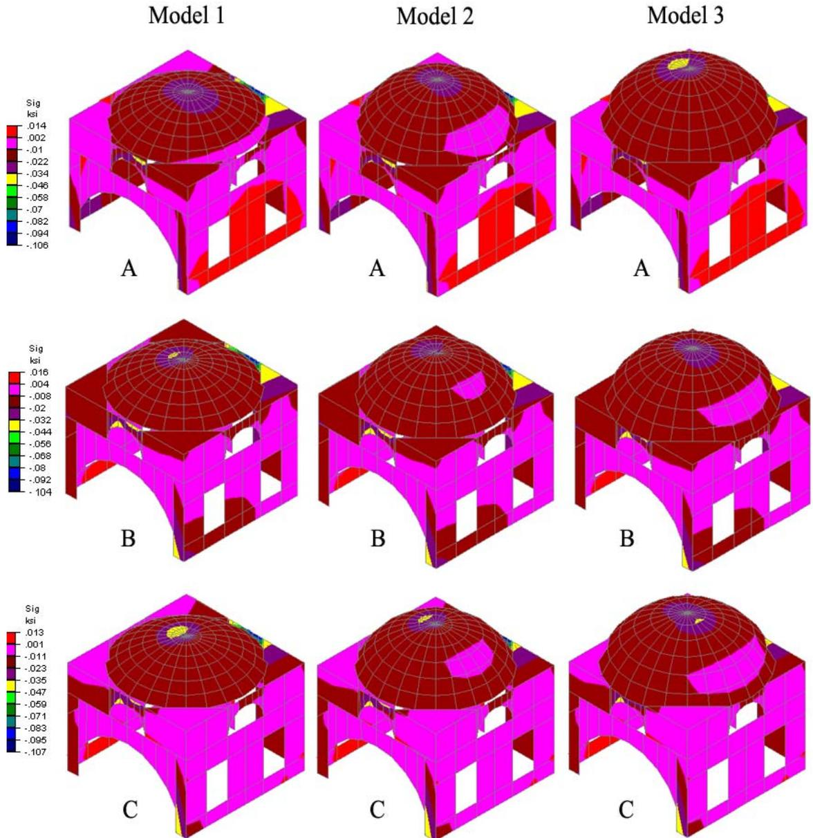
The stresses above are much lower than the allowable stresses and they are slightly over the values of the traditional bricks. This shows much better performance against traditional brick due to the comparison of the results and the allowable stresses. The shallow roof gets a larger stress than the other roofs.
