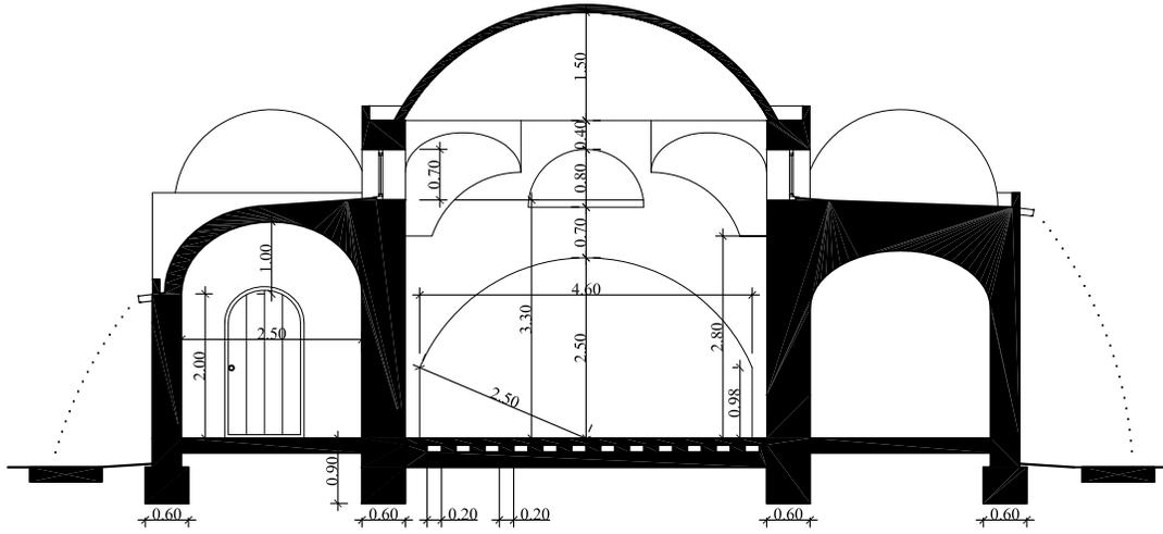
**FIG. 48 SINGLE UNIT A-A SECTION**
