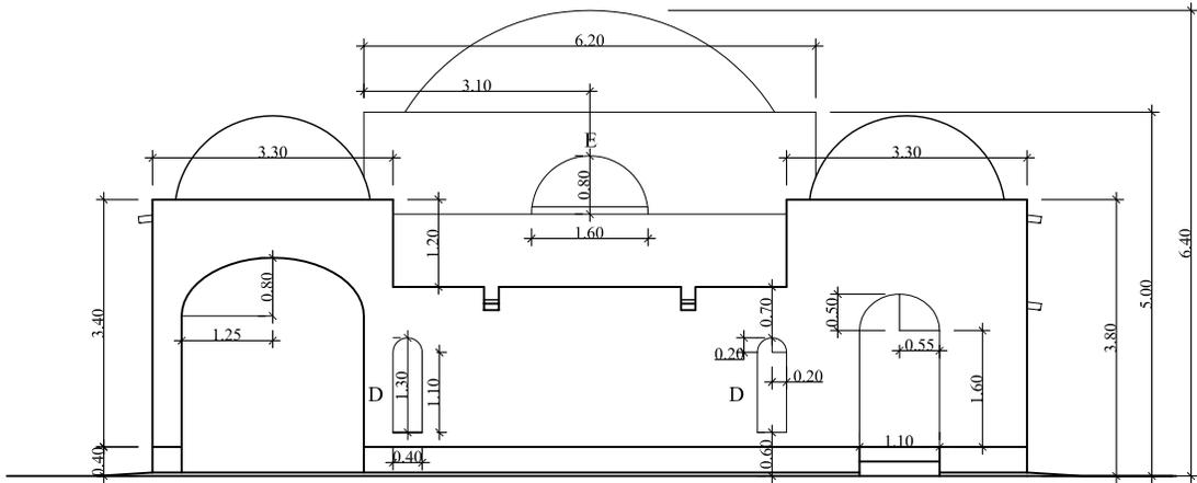
**FIG. 56** SINGLE UNIT DIMENSIONAL WEST ELEVATION
