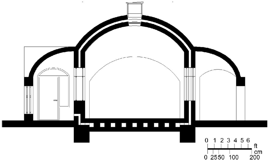
The unit is criticized for its unused spaces and lack of alternative space variations. Due to the relationship between the shape of the space and the roof type, use of the double dome is also criticized and it is suggested that the use of a vault would be appropriate if the space beneath is rectangular. Later on with the other proposal this idea lead to shape the main space.
