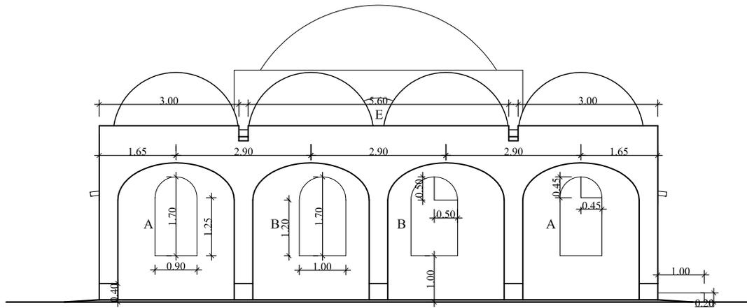
**FIG. 57** SINGLE UNIT DIMENSIONAL NORTH ELEVATION
