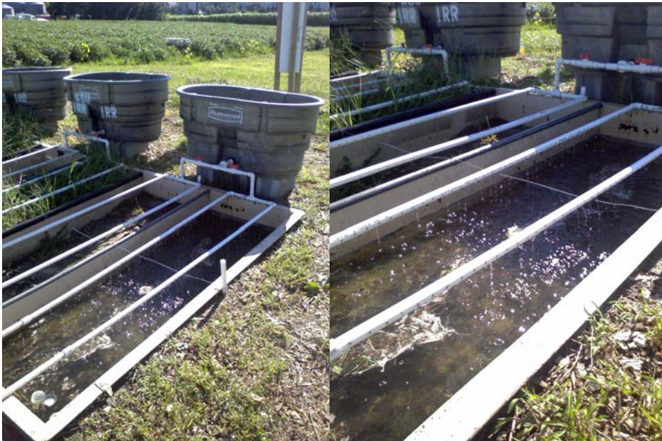
Figure 4.7 Stormwater ponding on control (cell 6) during the second stormwater event
