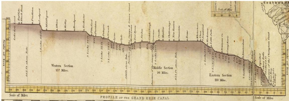
Figure 1. 1832 profile of the completed Erie Canal. The reasoning for beginning construction in the middle section is evident by its relatively small change in elevation compared to the western and eastern sections.
