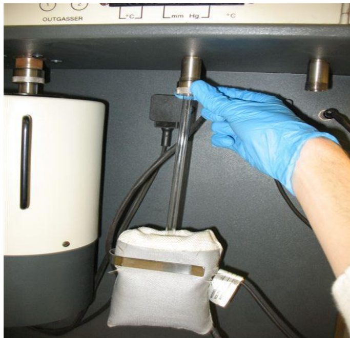
Figure 3-11: Final arrangement of bulb before out gassing.
