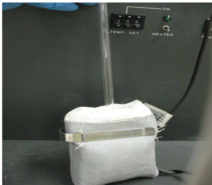
Figure 3-10: Bulb placed into the insulating heat bag.
