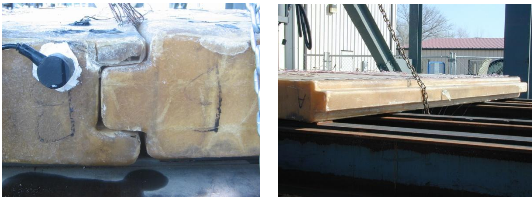
Figure 2-1 Tongue and Groove Connection (Left) & Tongue Edge (Right)
