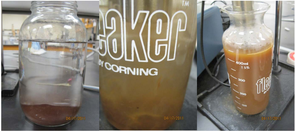
Figure 26. Magnetite in solution before, during, and after sonication from left to right.
