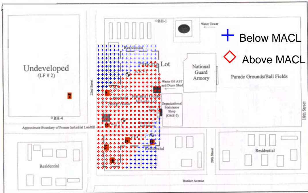
Figure 5.6. Distribution of copper in soil in regard to its MACL
