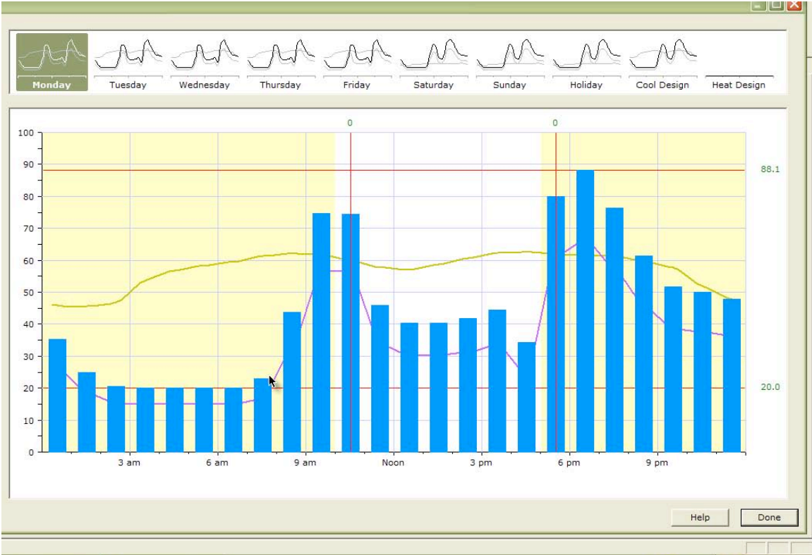
Figure C-41: Spring miscellaneous equipment profiles.
