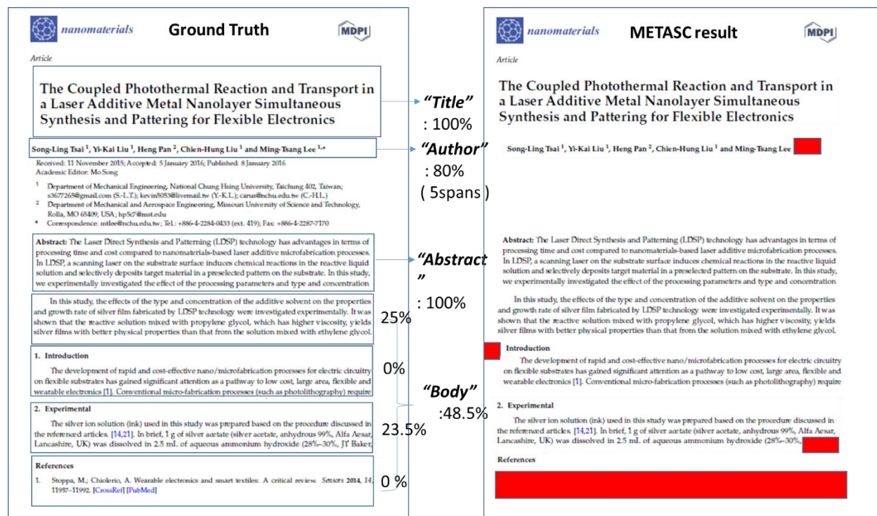
Figure 16. Example of the evaluation method for a document. The left shows ground truth while the right shows produced output of DBMATE. Here, for ‘introduction’ sub-subsection, the performance score is zero since one of the spans is missing.
