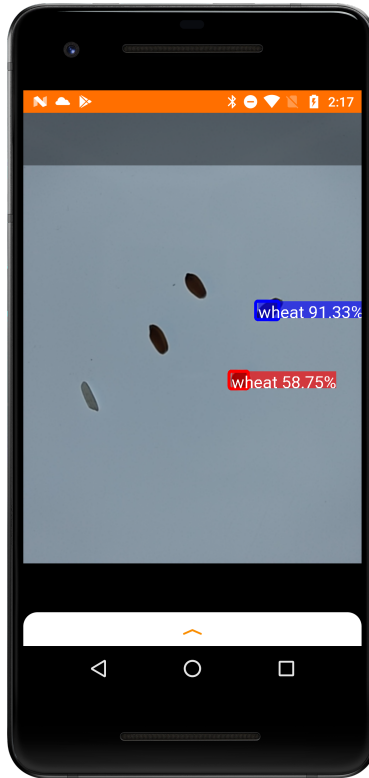
Figure 51: Application using SSDMobileNet to detect kernels.
