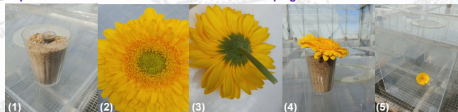
Figures: (1) 250 mL plastic cup with sand and 22 mL glass vial filled with water; (2) transvaal daisy flower; (3) transvaal daisy flower with excised stem; (4) transvaal daisy flower in glass vial with water; and (5) transvaal daisy flower in glass vial placed into 11.5 x 17.0 x 9.0 cm plexi-glass cage.
